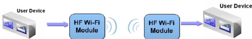
Figure 64. Transparent Serial Port Application
