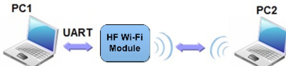
Figure 57. AP Interface Debug Connection
