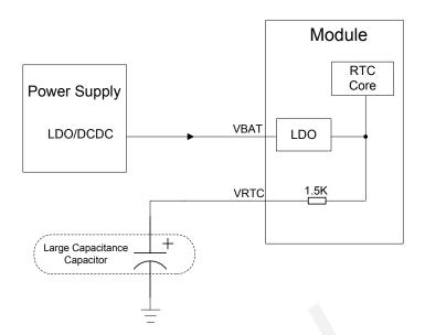
Figure 13: VRTC is Supplied by a Capacitor
