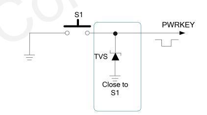
Figure 7: Turn on the Module with a Button
