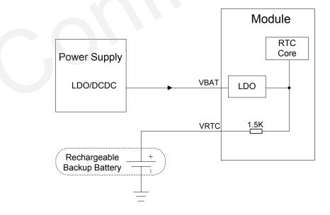
Figure 12: VRTC is Supplied by a Rechargeable Battery
