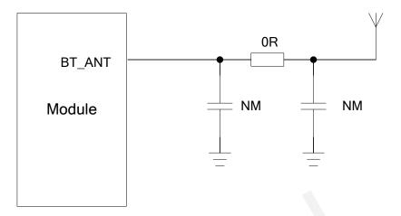
Figure 42: Reference Design for Bluetooth Antenna
