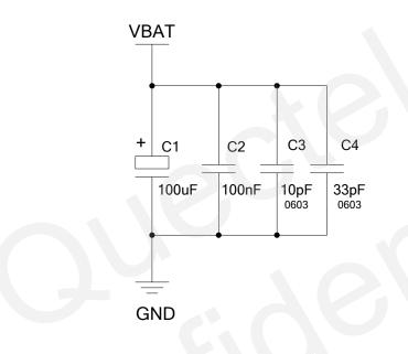
Figure 4: Reference Circuit for the VBAT Input
