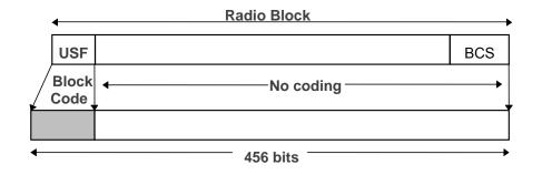
Figure 52: Radio Block Structure of CS-4
