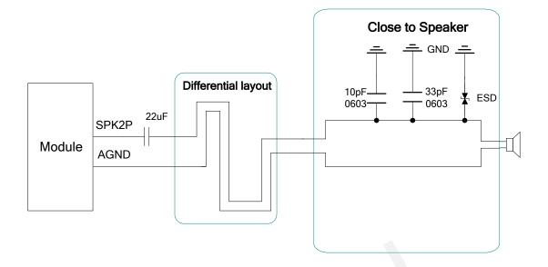
Figure 25: Handset Interface Design for AOUT2
