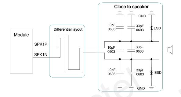
Figure 23: Handset Interface Design for AOUT1
