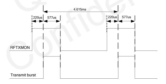
Figure 38: RFTXMON Signal during Burst Transmission
