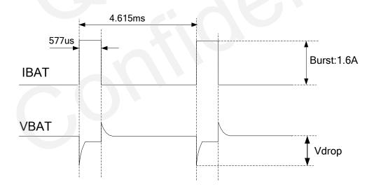
Figure 3: Voltage Ripple during Transmitting
