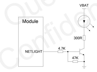
Figure 37: Reference Design for NETLIGHT
