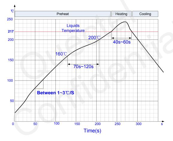
Figure 48: Ramp-Soak-Spike Reflow Profile
