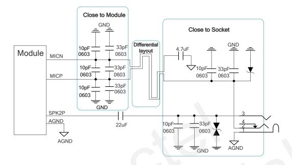
Figure 27: Earphone Interface Design
