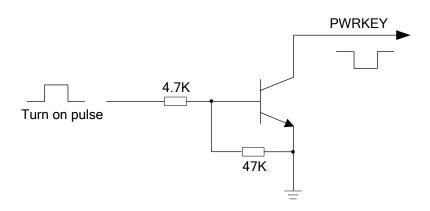
Figure 6: Turn on the Module with an Open-collector Driver
