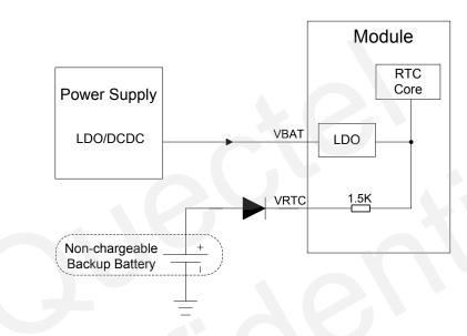
Figure 11: VRTC is Supplied by a Non-chargeable Battery
