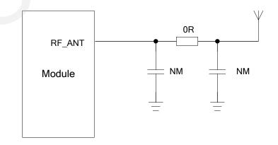
Figure 40: Reference Design for GSM Antenna
