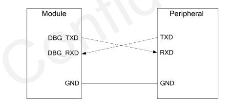
Figure 18: Reference Design for Debug Port
