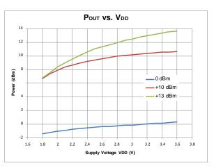
Figure 8. Output Power vs. Supply Voltages,  $F_{RF}$  = 433.92 MHz
