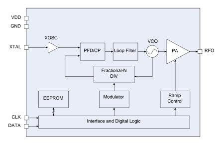
Figure 11. RFM119ABW/RFM119ACW Functional Block Diagram
