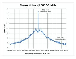
Figure 4. Phase Noise, F<sub>RF</sub> = 868.35 MHz,
