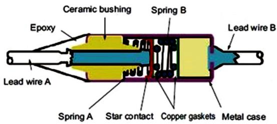
There is movable electrode, spring and thermal frit installed inside the RY-type thermal fuse. The spring B is installed under compressed condition, the spring force of which can hold the coppering gasket to keep the movable electrode well connected with the lead A. In normal condition, the current leads A, the movable electrode, the metal shell and wire B is conductive with each other.
