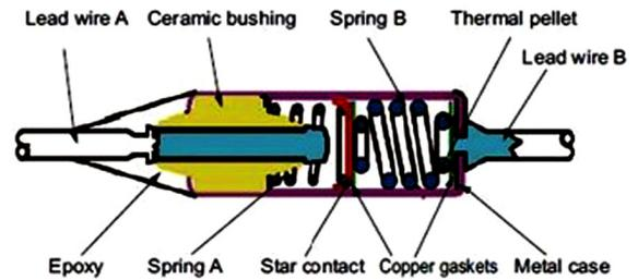
When the ambient temperature exceeds the operating temperature, the lead, the heat incoming from the lead and metal shell will melt thermal frit into liquid. At that time, the spring A and the spring B will popup and stretch, the elastic force of the spring A will push the movable electrode toward the spring B-side, so as to cut off contact with the leads A to cut off the circuit.
