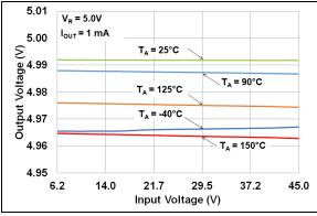
**FIGURE 2-2:** Output Voltage vs. Input Voltage ( $V_R = 5.0V$ ).
