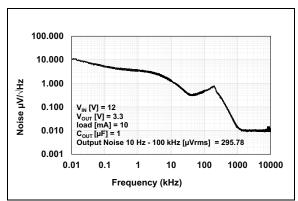
**FIGURE 2-14:** Noise vs. Frequency  $(V_R = 3.3V)$ .
