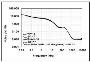
**FIGURE 2-15:** Noise vs. Frequency  $(V_R = 5.0V)$ .
