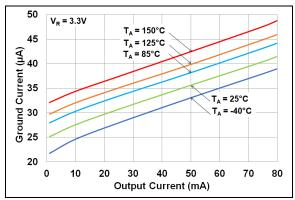
**FIGURE 2-12:** Ground Current vs. Output Current ( $V_R = 3.3V$ ).
