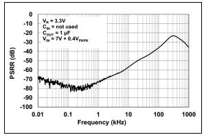
**FIGURE 2-16:** Power Supply Ripple Rejection Ratio vs. Frequency  $(V_R = 3.3V)$ .
