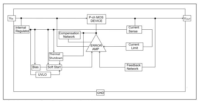
FIGURE 4-1: Simplified Functional Block Diagram.
