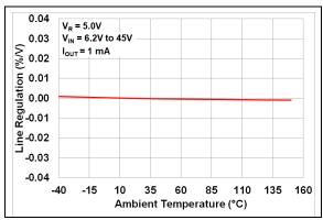
**FIGURE 2-9:** Line Regulation vs. Ambient Temperature ( $V_R = 5.0V$ ).
