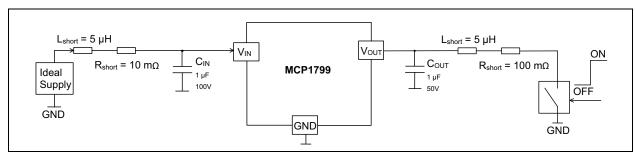
FIGURE 4-2: Short Circuit Test Set-Up.
