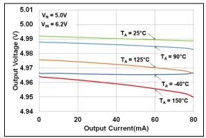
**FIGURE 2-4:** Output Voltage vs. Output Current ( $V_R = 5.0V$ ).
