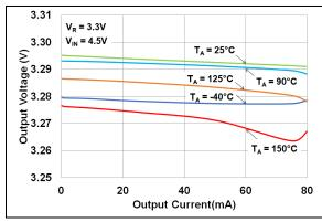
**FIGURE 2-3:** Output Voltage vs. Output Current ( $V_R = 3.3V$ ).
