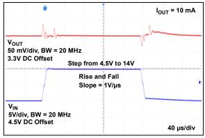
FIGURE 2-20: Line Step Response  $(V_R = 3.3V)$ .
