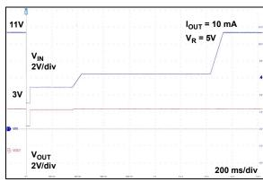
FIGURE 4-3: Line Step from Dropout.
