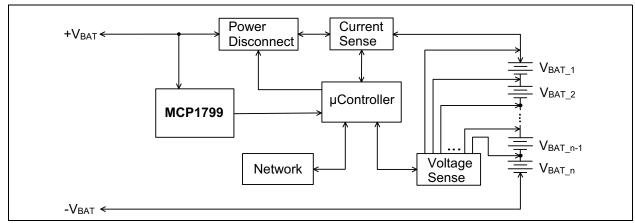
FIGURE 6-1: Smart Battery Pack Application Example.
