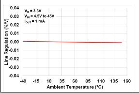
**FIGURE 2-8:** Line Regulation vs. Ambient Temperature ( $V_R = 3.3V$ ).
