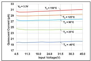
**FIGURE 2-10:** Quiescent Current vs.Input Voltage ( $V_R = 3.3V$ ).
