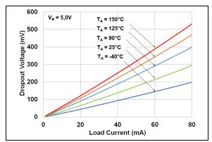
**FIGURE 2-5:** Dropout Voltage vs. Output Current.
