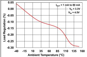
**FIGURE 2-6:** Load Regulation vs. Ambient Temperature ( $V_R = 3.3V$ ).
