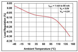
**FIGURE 2-7:** Load Regulation vs. Ambient Temperature  $(V_R = 5.0V)$ .
