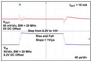
**FIGURE 2-21:** Line Step Response  $(V_R = 5.0V)$ .
