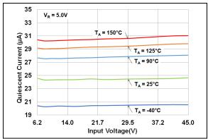
**FIGURE 2-11:** Quiescent Current vs.Input Voltage ( $V_R = 5.0V$ ).
