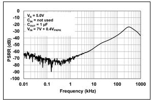
**FIGURE 2-17:** Power Supply Ripple Rejection Ratio vs. Frequency ( $V_R = 5.0V$ ).
