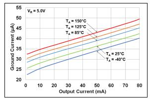
**FIGURE 2-13:** Ground Current vs. Output Current ( $V_R = 5.0V$ ).
