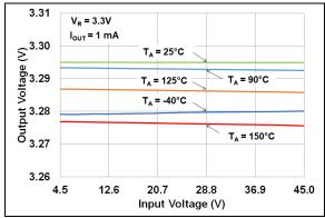
**FIGURE 2-1:** Output Voltage vs. Input Voltage  $(V_R = 3.3V)$ .
