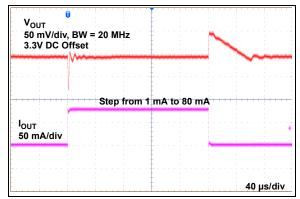
**FIGURE 2-18:** Load Step Response  $(V_R = 3.3V)$ .
