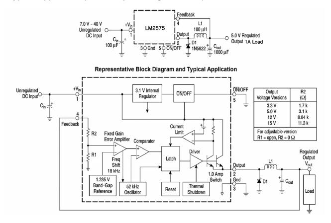
Figure 1. Block Diagram and Typical Application
