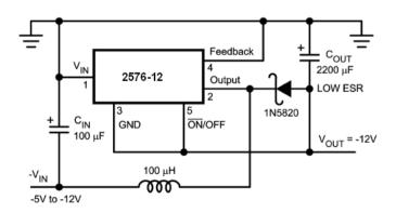
Typical Load Current 400 mA for VIN = -5.2V 750 mA for VIN = -7V Note: Heat sink may be required.
