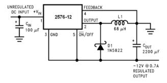
FIGURE 5. Inverting Buck-Boost Develops -12V
