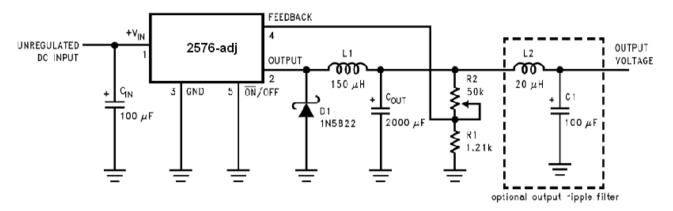
FIGURE 10. Adjustable 1A Power Supply with Low Output Ripple
