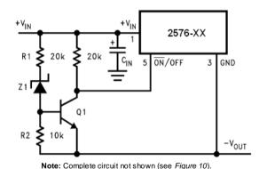
FIGURE 8. Undervoltage Lockout for Buck-Boost Circuit
