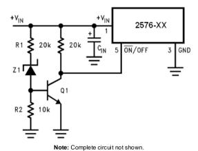
FIGURE 7. Undervoltage Lockout for Buck Circuit
