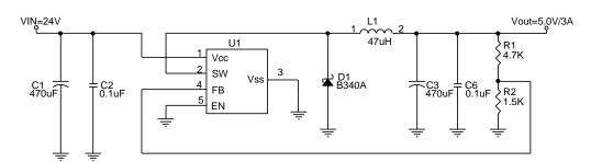
$$V_{OUT} = V_{FB} \times (1 + \frac{R1}{R2}), V_{FB} = 1.23V, R2 = 0.7K \sim 3K$$
