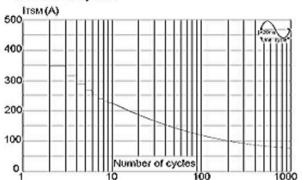
FIG.5: Non-repetitive surge peak on-state current for a sinusoidal pulse with width tp<20ms, and corresponging value of I't (dl/dt < 50A/μs)
