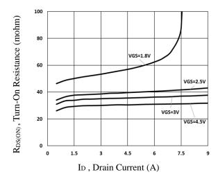
Fig.6 Turn-On Resistance vs. ID
