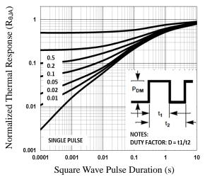
Fig.7 Normalized Transient Impedance
