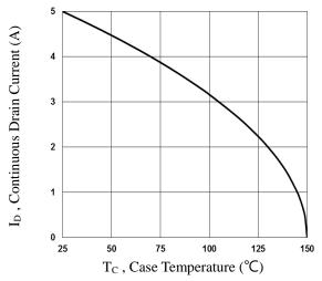
Fig.1 Continuous Drain Current vs. Tc
