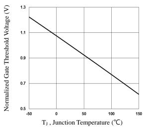
Fig.3 Normalized  $V_{th}$  vs.  $T_J$
