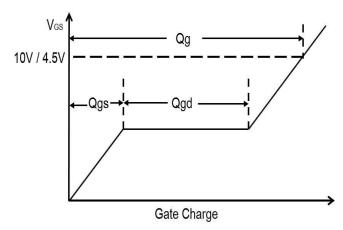
Fig.10 Gate Charge Waveform
