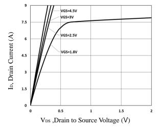
Fig.5 Typical Output Characteristics
