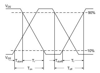
Fig.9 Switching Time Waveform
