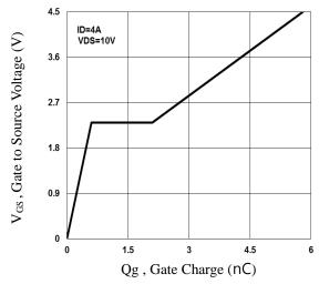
Fig.4 Gate Charge Waveform
