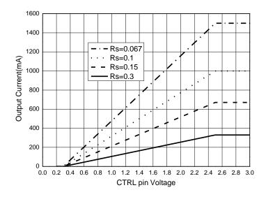
Figure 1. Analog Dimming Curve
