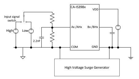
Figure 8-2. Common-Mode Transient Immunity Test Circuit
