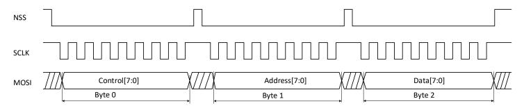
Figure 9-3. SPI Communication Protocol
