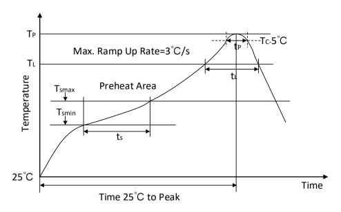
Figure 12-1. Soldering Temperature (reflow) Profile
