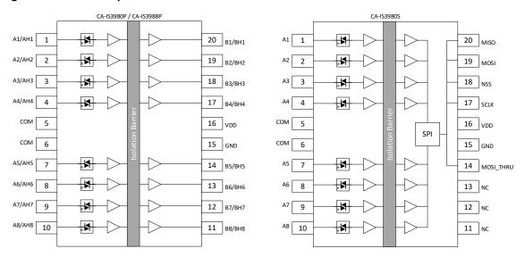
Figure 6-1. CA-IS398x Pin Configuration
