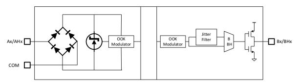
Figure 9-1. Simplified block diagram of a single CA-IS398x channel
