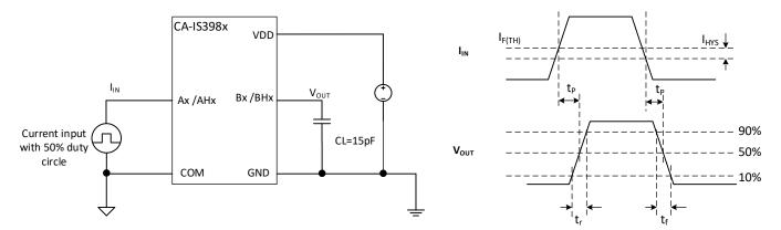
Figure 8-1. Switching Characteristics Test Circuit and Waveform
