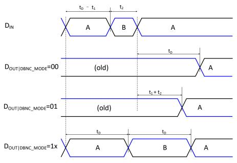
Figure 9-2. Debounce Filter Modes Timing Diagram
