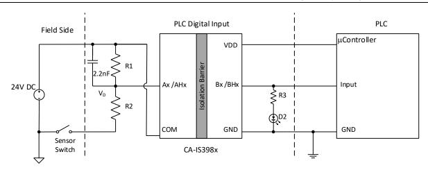
Figure 10-3. Typical Application Circuit with Sourcing Inputs
