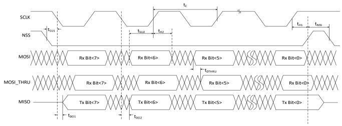
Figure 7-1. SPI Timing Diagram
