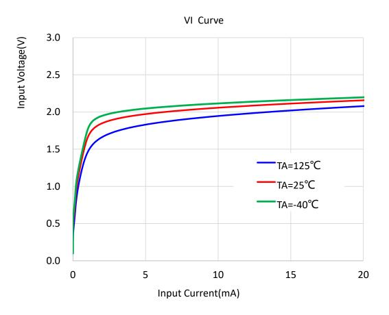
Figure 7-2. Input Voltage vs. Input Current Over Temperature
