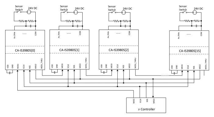
Figure 10-4. Typical Application Circuit with Daisy-Chaining
