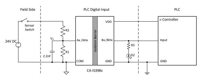
Figure 10-2. Typical Application Circuit with Sinking Inputs
