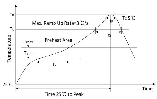
Figure 12-1 Soldering Temperature (reflow) Profile
