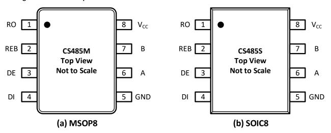
Figure 6-1. CS485 pin configuration
