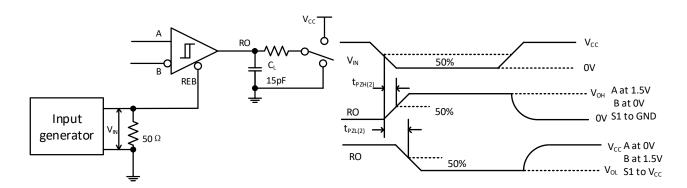
Figure 8-9. Receiver Enable Times With Driver Disabled
