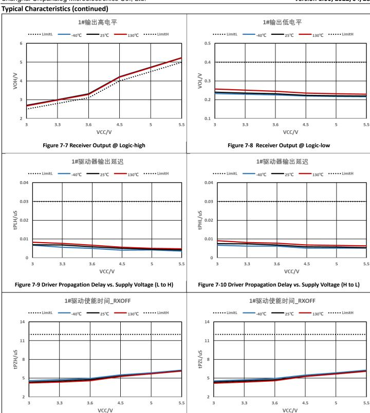
Figure 7-11 Driver Enable Time vs. Supply Voltage: tpzh
