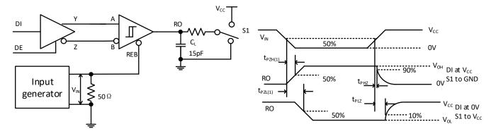
Figure 8-8. Receiver Enable/Disable Times With Driver Enabled
