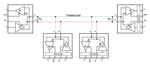
Figure 10-1. Typical RS-485 Network With CS485 Half-Duplex Transceivers
