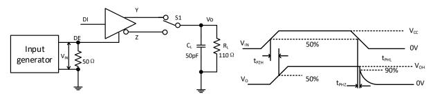
Figure 8-5. Driver Enable and Disable Times With Active High Output and Pull-Down Load
