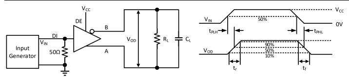
Figure 8-4 Driver Differential Output Rise and Fall Times and Propagation Delays
