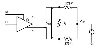
Figure 8-1. Driver Differential Output Voltage With Common-Mode Load
