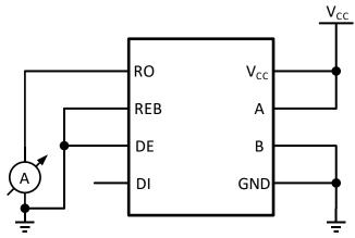
Figure 8-3. Receiver Output Short Current Measurement
