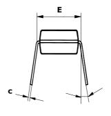
Note - Dimensions D, E1 do not include the fin value, which should not exceed 0.25 (0.010) per one side.
