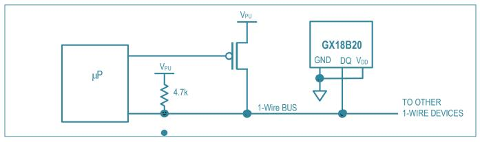
Figure 5. Powering the GX18B20 with an External Supply
