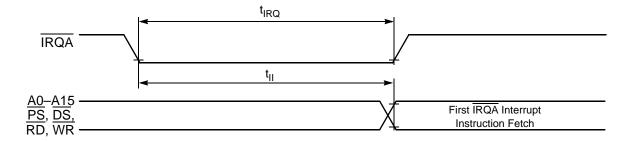
Figure 3-17 Recovery from Stop State Using IRQA Interrupt Service
