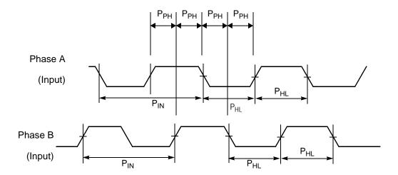
**Figure 3-24 Quadrature Decoder Timing**
