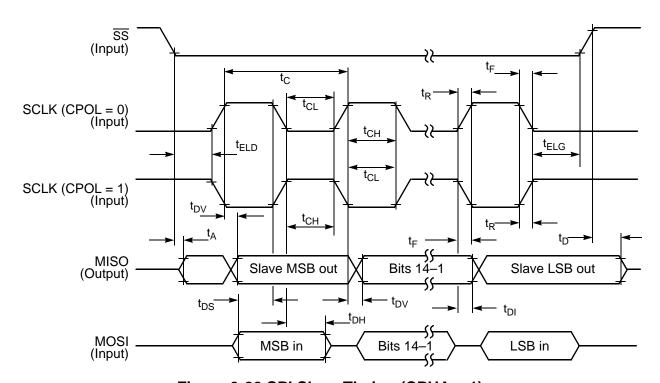
Figure 3-22 SPI Slave Timing (CPHA = 1)
