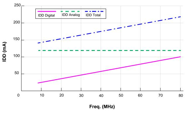
Figure 3-1 Maximum Run IDD vs. Frequency (see Note 6. in Table 3-14)
