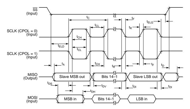
Figure 3-21 SPI Slave Timing (CPHA = 0)
