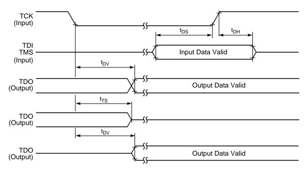
Figure 3-30 Test Access Port Timing Diagram
