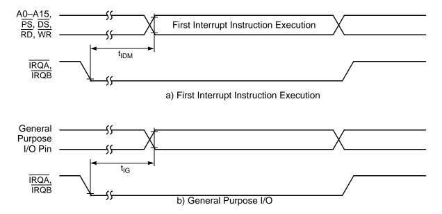
Figure 3-14 External Level-Sensitive Interrupt Timing
