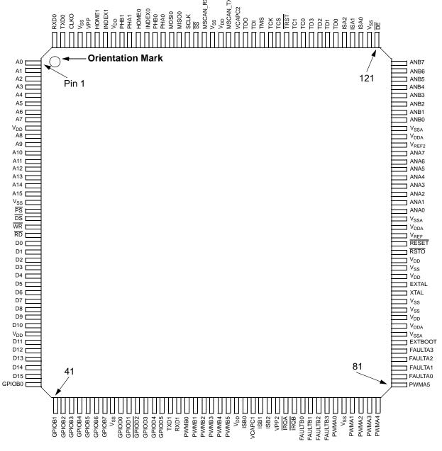
Figure 4-1 Top View, 56F807 160-pin LQFP Package
