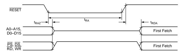
Figure 3-12 Asynchronous Reset Timing
