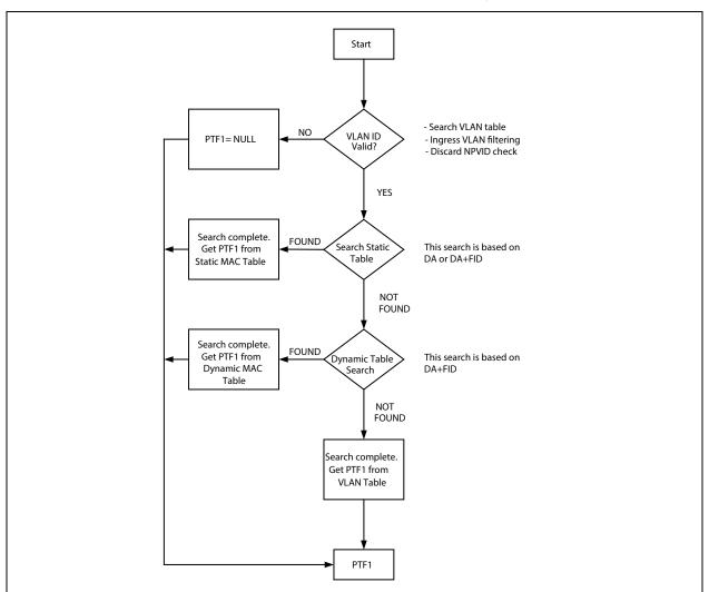
FIGURE 3-4: DESTINATION ADDRESS LOOKUP FLOW CHART, STAGE 1
