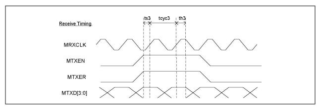
FIGURE 7-4: MAC MODE MII TIMING - DATA TRANSMITTED TO MII
