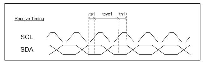
FIGURE 7-2: EEPROM INTERFACE OUTPUT TIMING DIAGRAM
