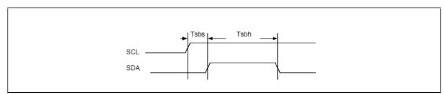
FIGURE 7-12: I<sup>2</sup>C OUTPUT TIMING
