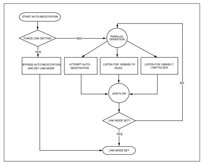
FIGURE 3-3: AUTO-NEGOTIATION AND PARALLEL OPERATION
