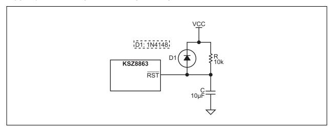
Figure 8-2 shows a reset circuit recommended for applications where reset is driven by another device (for example, the CPU or an FPGA). At power-on-reset, R, C, and D1 provide the necessary ramp rise time to reset the KSZ8863MLL/FLL/RLL device. The RST\_OUT\_N from the CPU/FPGA provides the warm reset after power-up.
