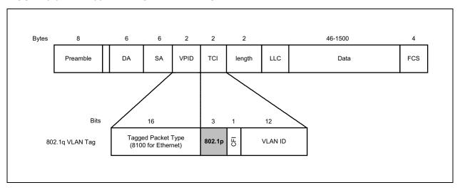
The 802.1p-based priority is enabled with bit [5] of registers 16, 32, and 48 for ports 1, 2, and 3, respectively.
