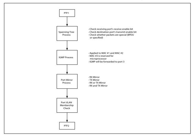
FIGURE 3-5: DESTINATION ADDRESS RESOLUTION FLOW CHART, STAGE 2
