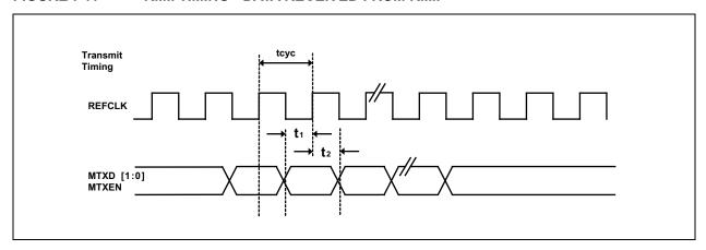
FIGURE 7-8: RMII TIMING - DATA TRANSMITTED TO RMII
