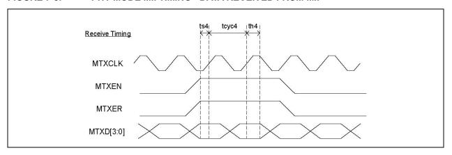
FIGURE 7-6: PHY MODE MII TIMING - DATA TRANSMITTED TO MII
