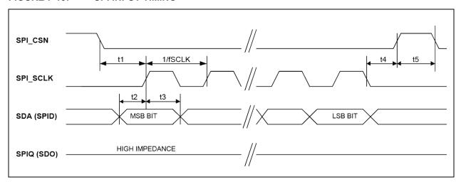
FIGURE 7-14: SPI OUTPUT TIMING
