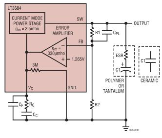
Figure 2. Model for Loop Response
