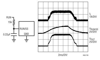
Figure 6. To Soft-Start the LT3684, Add a Resistor and Capacitor to the RUN/SS Pin
