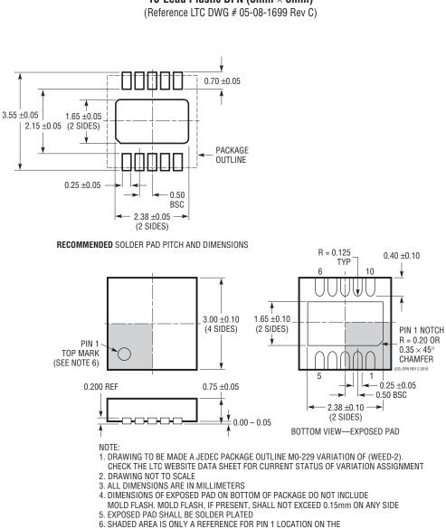
DD Package 10-Lead Plastic DFN (3mm × 3mm) (Reference LTC DWG # 05-08-1699 Rev C)
