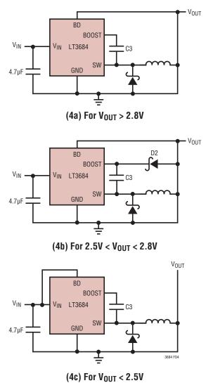
Figure 4. Three Circuits For Generating The Boost Voltage
