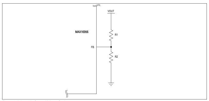
Figure 1. Adjustable Output-Voltage Setting
