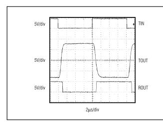
Figure 9. Loopback Test Result at 120kbps
