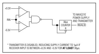
Figure 2a. Entering 1µA Supply Mode via AutoShutdown
