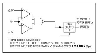
Figure 2b. Transmitter Enabled Using AutoShutdown
