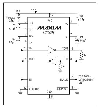
Figure 1. Shutdown Current Test Circuit
