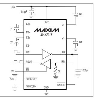
Figure 8. Loopback Test Circuit
