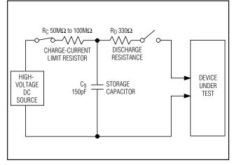
Figure 6a. IEC 1000-4-2 ESD Test Model
