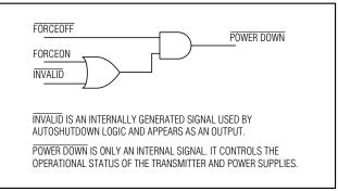
Figure 2c. AutoShutdown Logic
