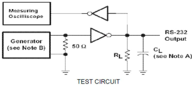
Maximum Data Rate Test Circuit
