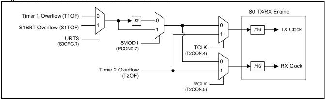
When S1BRG is used as the baud rate generator of S0, the baud rate is as follows.
