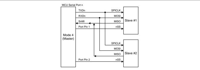
The SPI master satisfies the transfer with the full function SPI module of Megawin MG82/84 series MCU with CPOL, CPHA and DORD selection. For CPOL and CPHA condition, **MG82F6D64/32** uses an easy way by initialize SPI clock assigned port pin (TXD0) polarity to fit them. Table 18–41 shows the serial port Mode 4 mapping with the four SPI operating mode.
