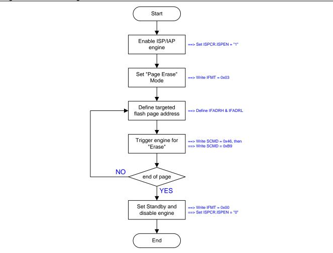
Figure 32-4 shows the demo code of the ISP/IAP page erase operation.
