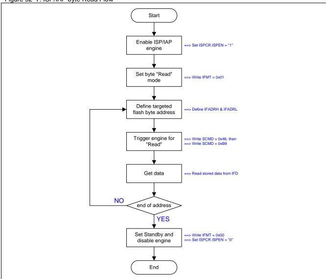
Figure 32–8 shows the demo code of the ISP/IAP byte read operation.
