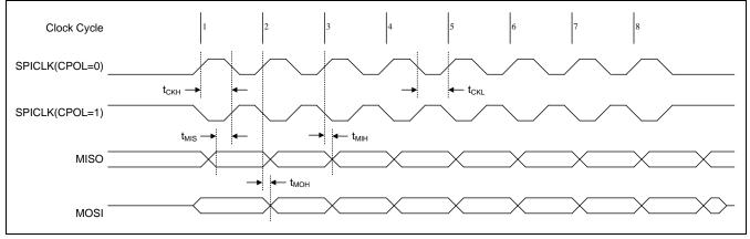
Figure 37–5. SPI Slave Transfer Waveform with CPHA=0
