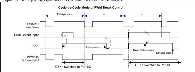
Bit 4~3: PBKE1.1~0, PWM Break Enable 1 selection. This function is only active on CEXn output mode (n=0~5).
