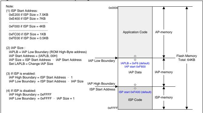
Figure 32–2. MG82F6D32 Flash Memory Configuration
