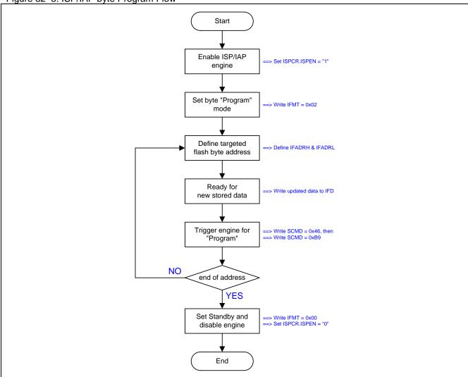
Figure 32-6 shows the demo code of the ISP/IAP byte program operation.
