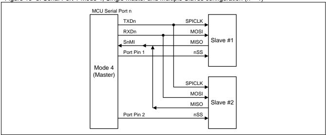
The SPI master satisfies the transfer with the full function SPI module of Megawin MG82/84 series MCU with CPOL, CPHA and DORD selection. For CPOL and CPHA condition, MG82F6D64/32 uses an easy way by initialize SPI clock polarity to fit them. Table 18–13 shows the serial port Mode 4 mapping with the four SPI operating mode.
