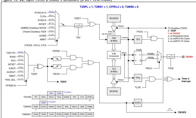
Figure 16-22. Split Timer 2 Mode 4 Structure (8-bit PWM mode)
