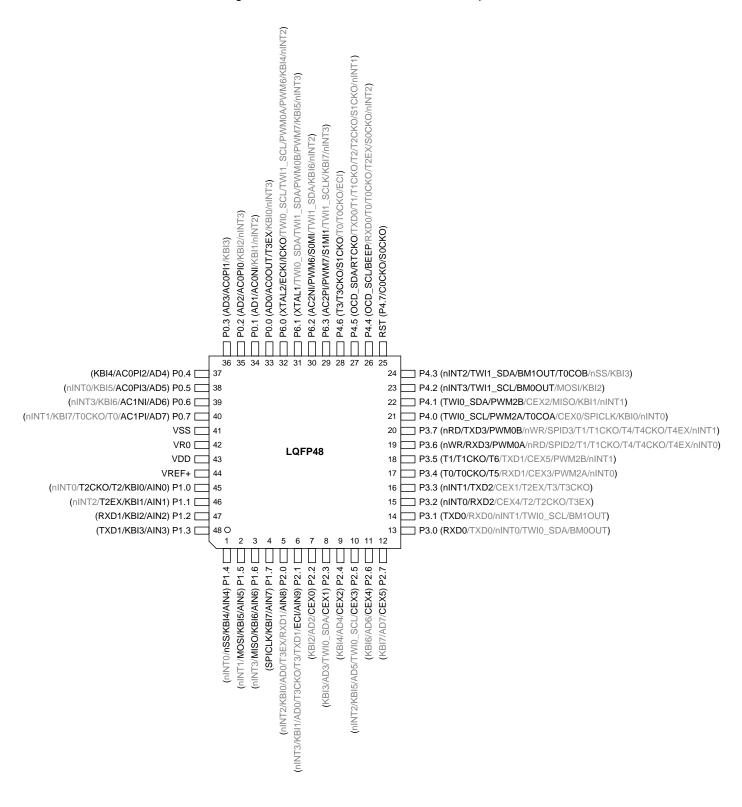
Figure 4-3. MG82F6D32AD48 LQFP48 Top View
