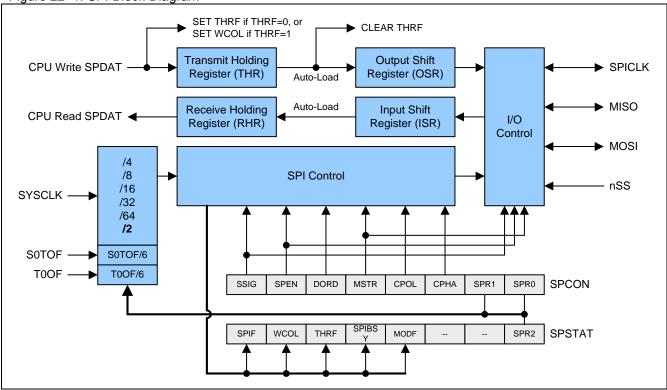
The SPI interface has four pins: MISO, MOSI, SPICLK and nSS:
