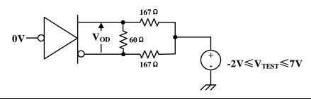
Fig.3 Driver Vod test circuit
