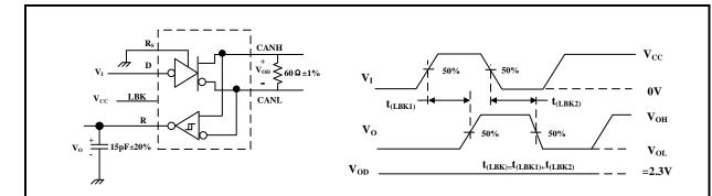
The input pulse is supplied by a generator having the following characteristics: PRR=125kHz, 50% duty cycle,  $t_r$ <6ns,  $t_f$ <6ns.
