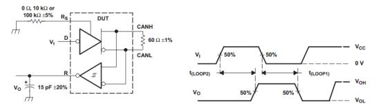
The input pulse is supplied by a generator having the following characteristics: PRR $\leq$ 125kHz, 50% duty cycle,  $t_r$ <6ns,  $t_f$ <6ns, Zo=50 $\Omega$ .
