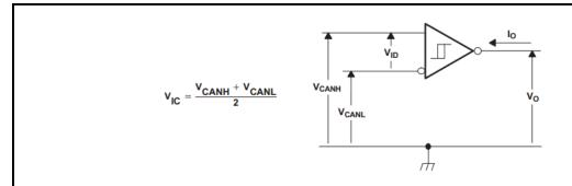
Fig.5 Receiver voltage and current definitions
