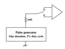
A, D, RS, LBK input state is 0 or  $V_{\text{CC}}$ .
