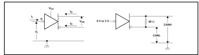
Fig.1 Driver voltage, current and test definition
