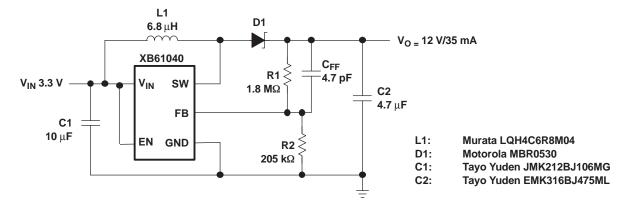
Figure 20. Standard 3.3-V to 12-V Supply
