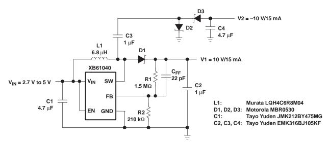
Figure 19. Positive and Negative Output LCD Bias Supply
