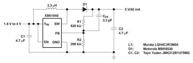
Figure 21. Dual Battery Cell to 5-V/50-mA Conversion Efficiency Approx. Equals 84% at  $V_{\rm IN}$  = 2.4 V to Vo = 5 V/45 mA
