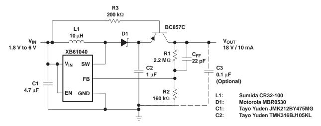
Figure 18. LCD Bias Supply With Load Disconnect
