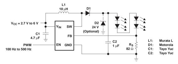
Figure 22. White LED Supply With Adjustable Brightness Control Using a PWM Signal on the Enable Pin, Efficiency Approx. Equals 86% at  $V_{\rm IN}$  = 3 V,  $I_{\rm LED}$  = 15 mA
