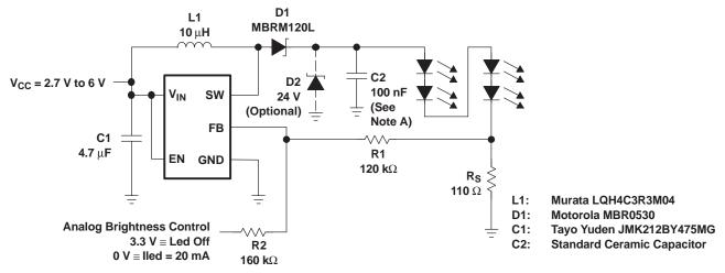
A. A smaller output capacitor value for C2 causes a larger LED ripple.
