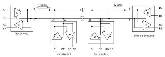
Figure 9. Typical Half-Duplex RS-485 Network
