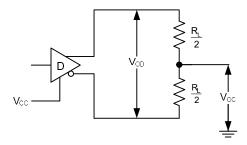
Figure 1. Driver  $V_{\text{OD}}$  and  $V_{\text{OC}}$
