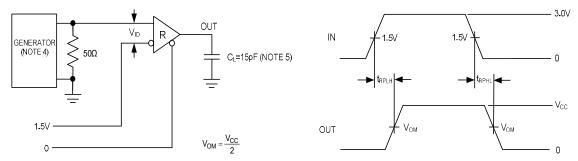
Figure 7. Receiver Propagation Delay
