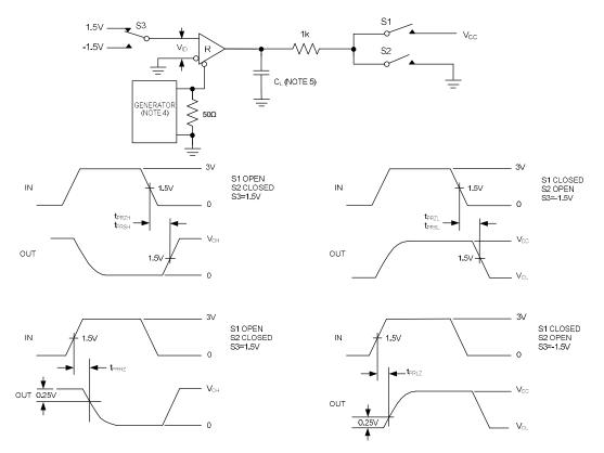
Figure 8. Receiver Enable and Disable Times
