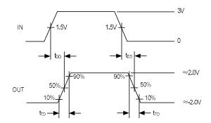
Figure 3. Driver Differential Output Delay and Transition Times
