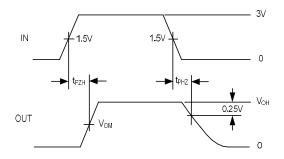
Figure 5. Driver Enable and Disable Times (t<sub>PZH</sub>, t<sub>PSH</sub>, t<sub>PHZ</sub>)
