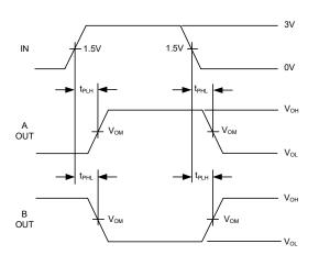
Figure 4. Driver Propagation Times
