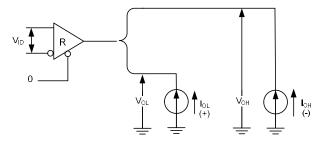
Figure 2. Receiver  $V_{\text{OH}}$  and  $V_{\text{OL}}$
