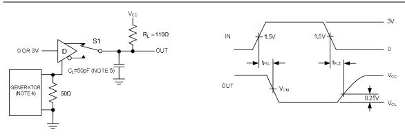
Figure 6. Driver Enable and Disable Times (tpzl, tpsl, tplz)
