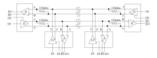
Figure 2: Typical Full-Duplex RS-422 Network
