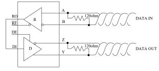
Figure 11. Receiver Propagation Delay Test Circuit
