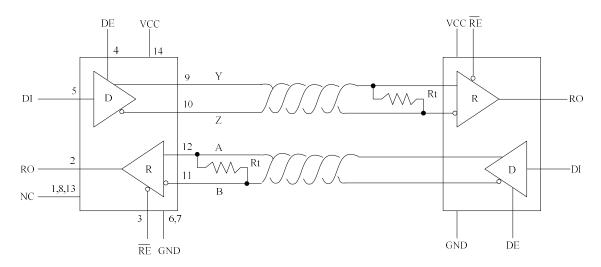
Figure 1: UM3491 pin configuration and typical full-duplex operating circuit
