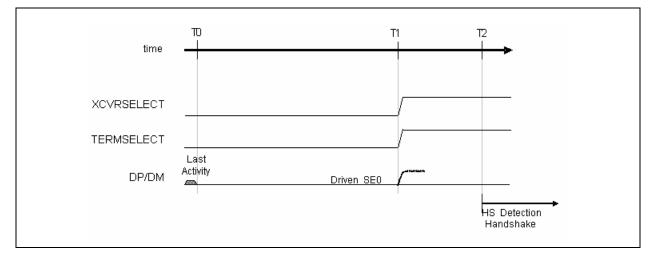
FIGURE 8-1: RESET TIMING BEHAVIOR (HS MODE)
