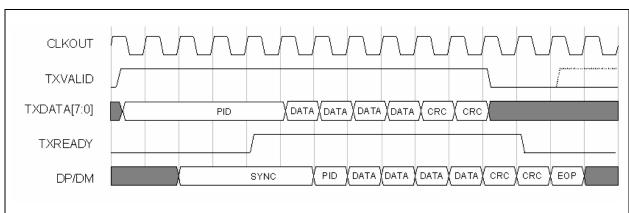
FIGURE 7-3: TRANSMIT TIMING FOR A DATA PACKET
