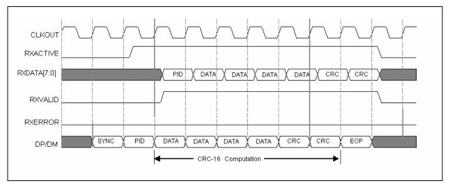
FIGURE 7-7: RECEIVE TIMING FOR DATA PACKET (WITH CRC-16)
