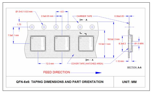
FIGURE 9-2: QFN, 6X6 TAPE & REEL
