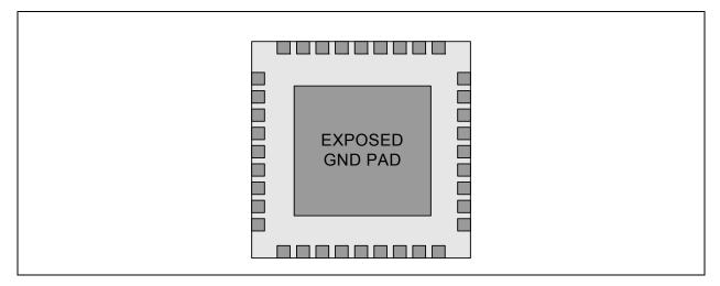
The flag of the QFN package must be connected to ground.
