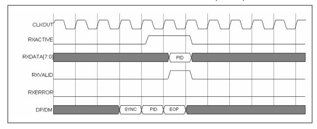
FIGURE 7-6: RECEIVE TIMING FOR SETUP PACKET
