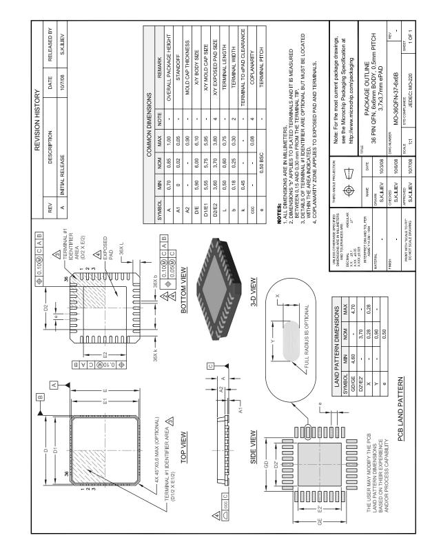
FIGURE 9-1: USB3280-AEZG 36-PIN QFN PACKAGE OUTLINE AND PARAMETERS, 6 X 6 X 0.90 MM BODY (ROHS COMPLIANT)
