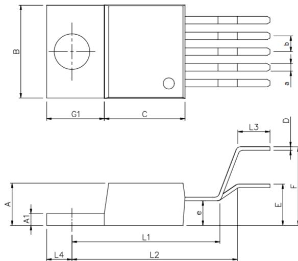
Dimensions In Millimeters(TO220B-5)
