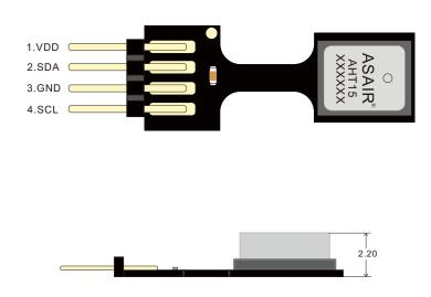
Figure 1: AHT15 Sensor Package Diagram (Unit: mm Tolerance: 0.1 mm)
