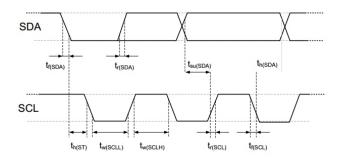
Figure 9.The sequence diagrams and abbreviations of digital input/output are explained in Table 8. Thicker SDA lines are controlled by sensors, and ordinary SDA lines are controlled by single chip computer. Please be noted that the effective read time of SDA is triggered by the drop edge of the previous conversion
