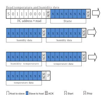
Note: The sensor takes time to collect data. After the host sends out the measurement command (0 xAC), it delays more than 75 milliseconds to read the converted data and judge whether the returned status bits are normal. If the state bit [Bit 7] is 0, the data can be read normally, and 1 represents that the sensor is busy, the host needs to wait for data processing to complete.
