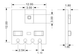
Figure 13. AHT21B sensor encapsulation (unit: mm not specified tolerance: ± 0.2 mm)
