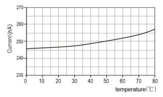
Figure 6. Typical supply current vs. temperature curve (sleep mode) when VDD=3.3V
