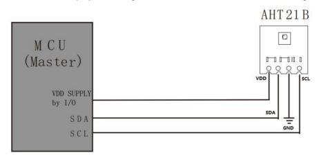
Figure 8. Typical application circuit
