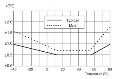
Figure 3. Typical and maximum temperature errors
