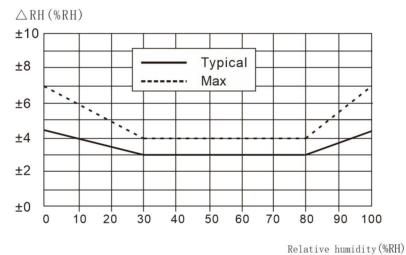
Figure 2. Typical and maximum humidity errors
