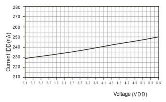
Figure 7. The relationship between current and voltage at 25℃
