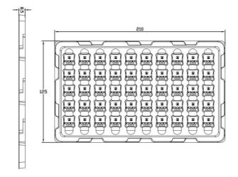
Figure 12. ATH21B sensor package diagram (unit: mm unmarked tolerance: ± 0.2mm)
