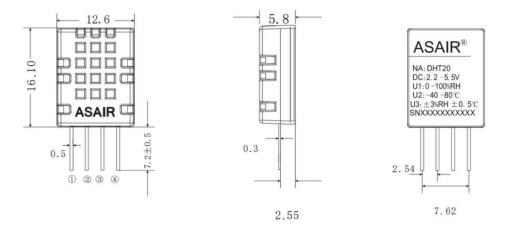
Figure 13. DHT20 sensor encapsulation (unit: mm not specified tolerance: ± 0.2 mm)
