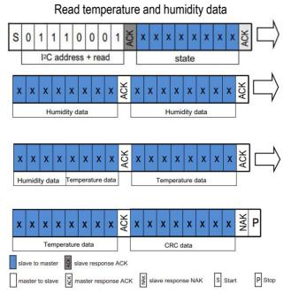
Note: The sensor needs time to collect. After the host sends a measurement command (0xAC), delay more than 80 milliseconds before reading the converted data and judging whether the returned status bit is normal. If the status bit [Bit7] is 0, it means that the data can be read normally. When it is 1, the sensor is busy, and the host needs to wait for the data processing to complete.
