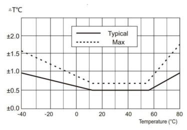
Figure 3. Typical and maximum temperature errors
