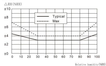
Figure 2. Typical and maximum humidity errors
