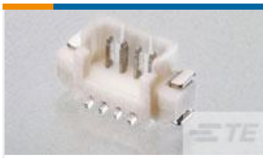
TE Part #1734260-4 1.25 WTB HDR SMT, 4 POS
