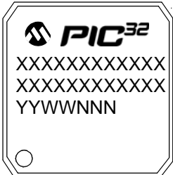
100-Lead TQFP (12x12x1 mm)
