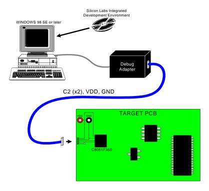
Figure 1.5. Development/In-System Debug Diagram
