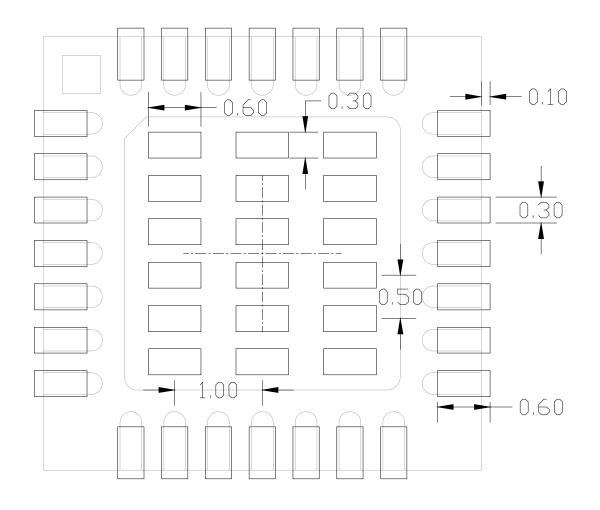
Figure 4.6. Typical QFN-28 Solder Paste Diagram
