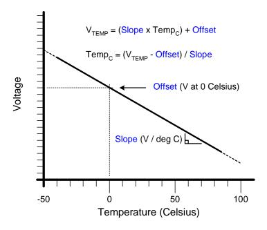
**Figure 8.2. Single Channel Transfer Function**
