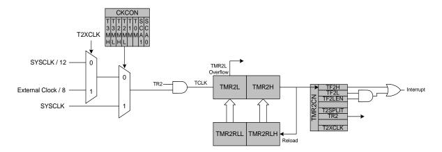
Figure 22.4. Timer 2 16-Bit Mode Block Diagram
