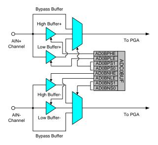
Figure 5.2. ADC0 Buffer Control
