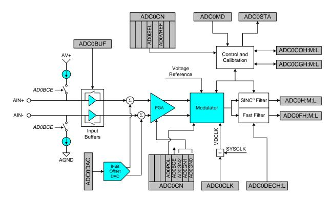
Figure 5.1. ADC0 Block Diagram
