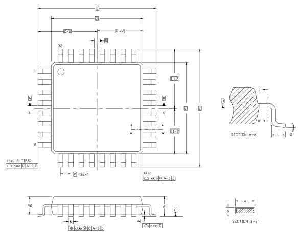
Figure 4.3. LQFP-32 Package Diagram
