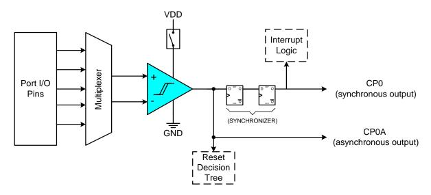
Figure 1.9. Comparator Block Diagram
