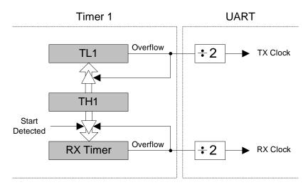
Figure 20.2. UARTO Baud Rate Logic
