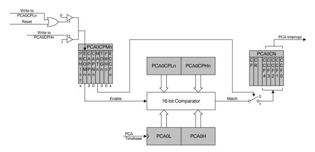
Figure 23.5. PCA Software Timer Mode Diagram
