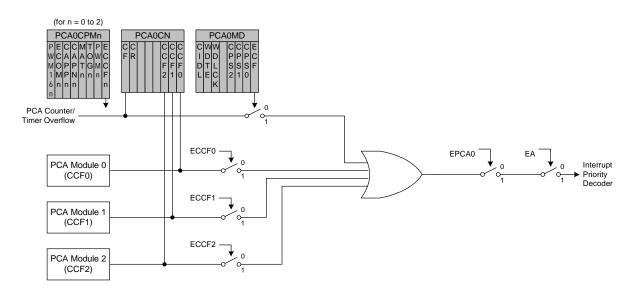
Figure 23.3. PCA Interrupt Block Diagram
