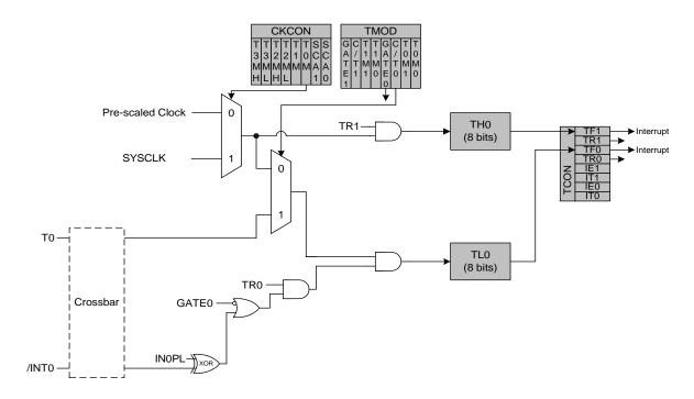
Figure 22.3. T0 Mode 3 Block Diagram
