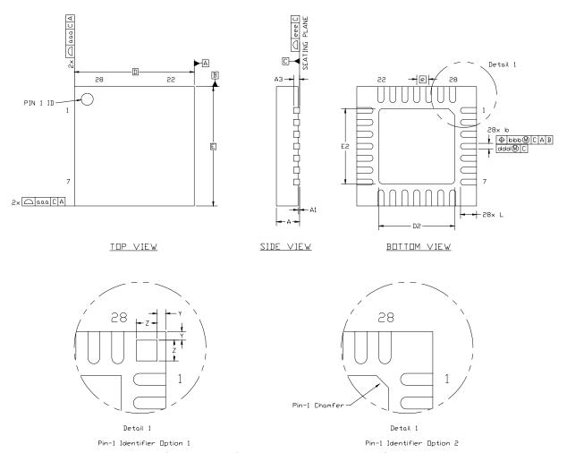
Figure 4.4. QFN-28 Package Drawing
