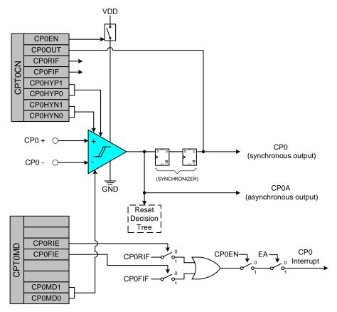
Figure 9.1. Comparator Functional Block Diagram
