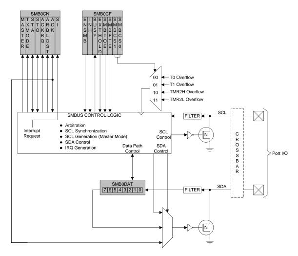
Figure 19.1. SMBus Block Diagram
