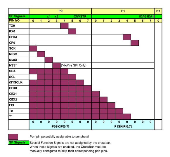
Figure 18.3. Crossbar Priority Decoder with No Pins Skipped
