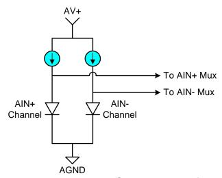
Figure 8.1. Temperature Sensor Block Diagram
