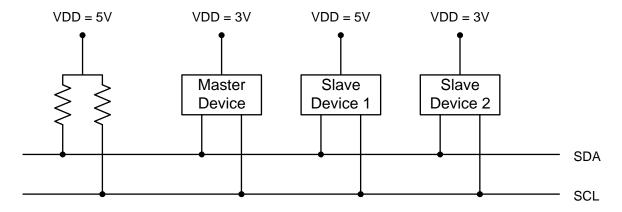
Figure 19.2. Typical SMBus Configuration
