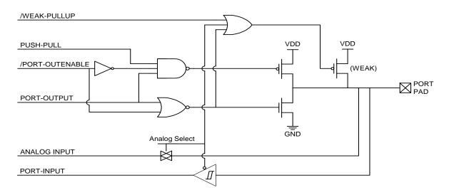
Figure 18.2. Port I/O Cell Block Diagram
