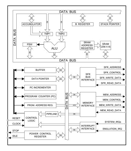
Figure 10.1. CIP-51 Block Diagram
