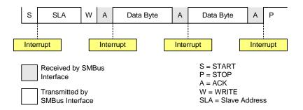
Figure 19.5. Typical Master Transmitter Sequence
