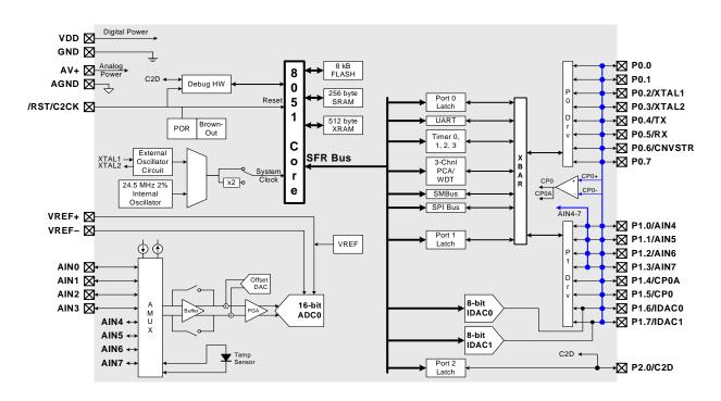
Figure 1.4. C8051F353 Block Diagram
