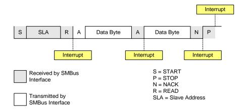
Figure 19.8. Typical Slave Transmitter Sequence
