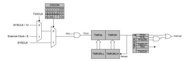
Figure 22.6. Timer 3 16-Bit Mode Block Diagram
