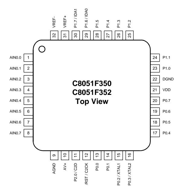
Figure 4.1. LQFP-32 Pinout Diagram (Top View)
