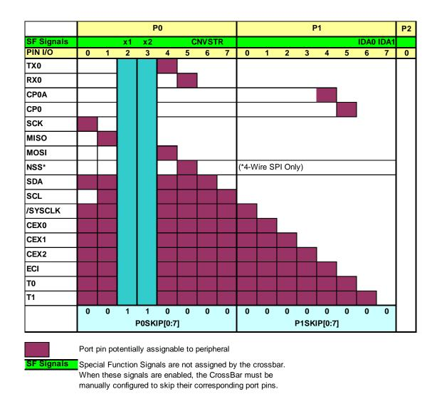
Figure 18.4. Crossbar Priority Decoder with Crystal Pins Skipped
