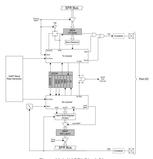
Figure 20.1. UARTO Block Diagram
