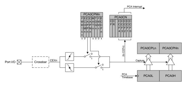
Figure 23.4. PCA Capture Mode Diagram
