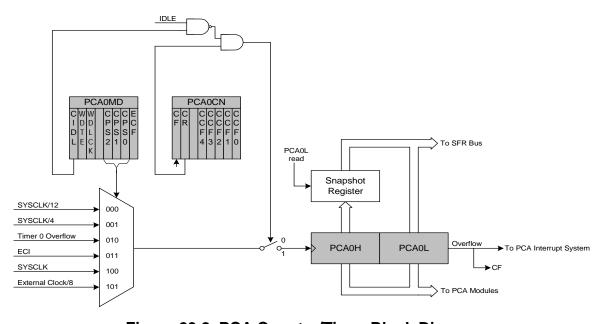
Figure 23.2. PCA Counter/Timer Block Diagram
