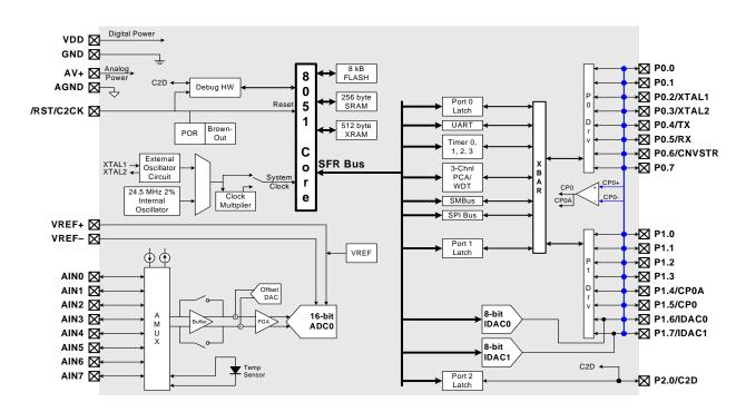
Figure 1.3. C8051F352 Block Diagram
