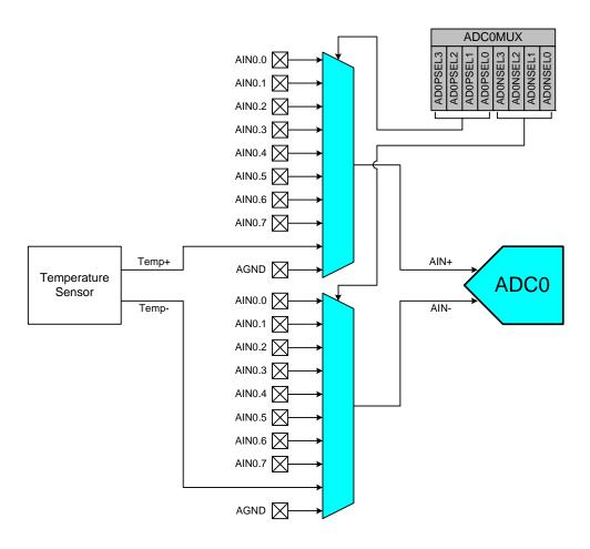
Figure 5.5. ADC0 Multiplexer Connections
