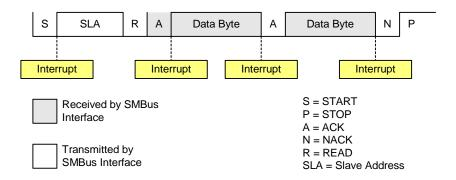
Figure 19.6. Typical Master Receiver Sequence
