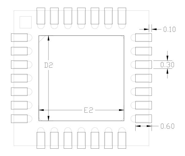
Figure 4.5. Typical QFN-28 Landing Diagram
