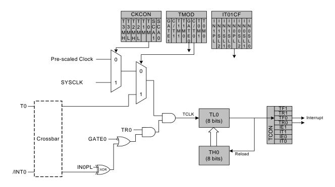
Figure 22.2. T0 Mode 2 Block Diagram
