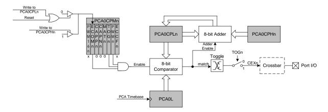
Figure 23.7. PCA Frequency Output Mode
