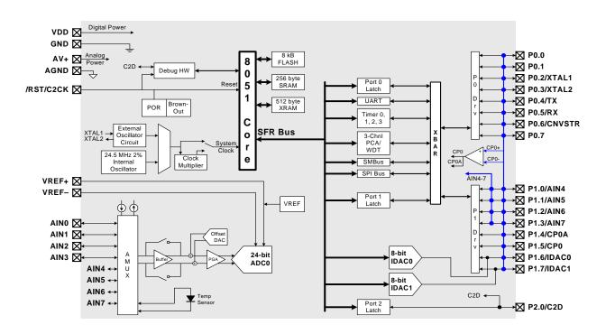
Figure 1.2. C8051F351 Block Diagram
