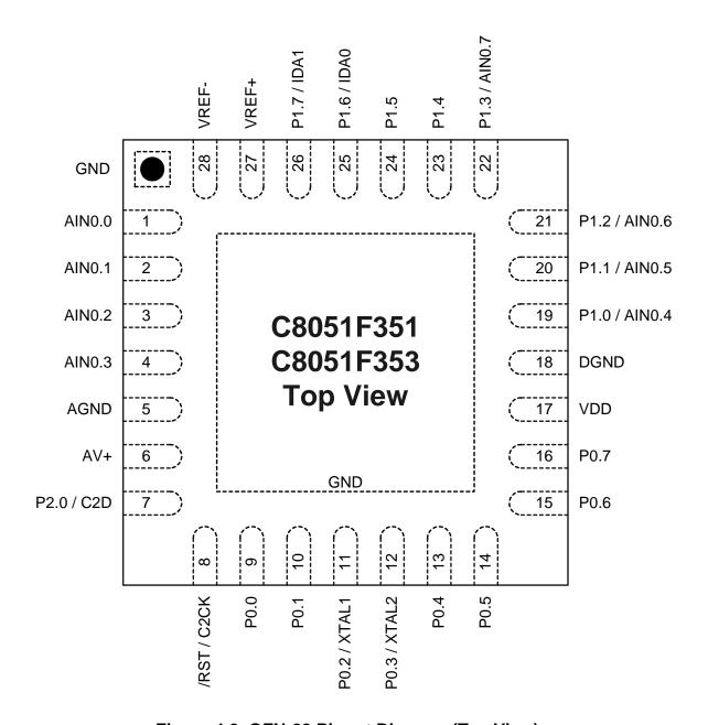
Figure 4.2. QFN-28 Pinout Diagram (Top View)
