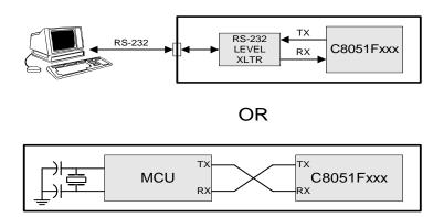
Figure 20.3. UART Interconnect Diagram
