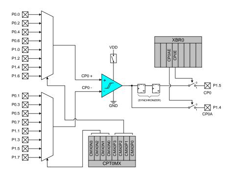
Figure 9.3. Comparator Pin Connections
