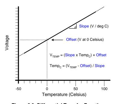
**Figure 8.3. Differential Transfer Function**
