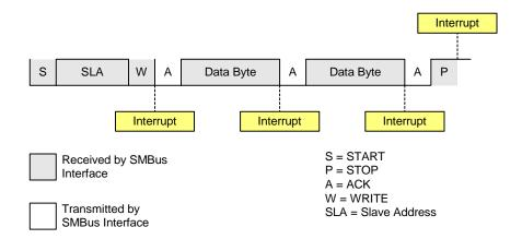
Figure 19.7. Typical Slave Receiver Sequence
