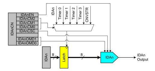
Figure 6.1. IDAC Functional Block Diagram
