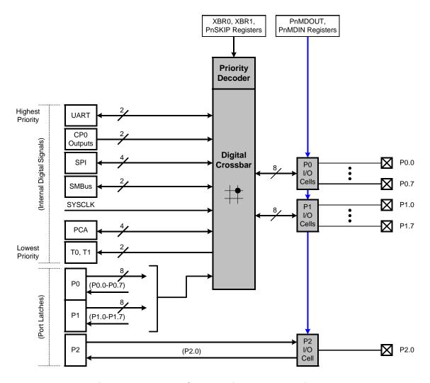
Figure 1.10. Port I/O Functional Block Diagram
