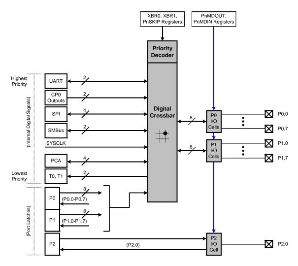
Figure 18.1. Port I/O Functional Block Diagram
