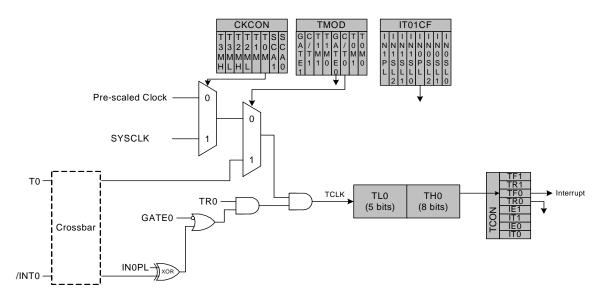
Figure 22.1. T0 Mode 0 Block Diagram
