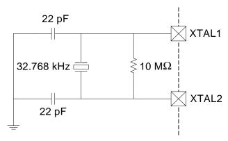
Figure 17.2. 32.768 kHz External Crystal Example
