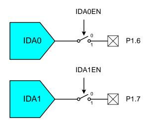
Figure 6.3. IDAC Pin Connections
