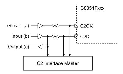
Figure 25.1. Typical C2 Pin Sharing
