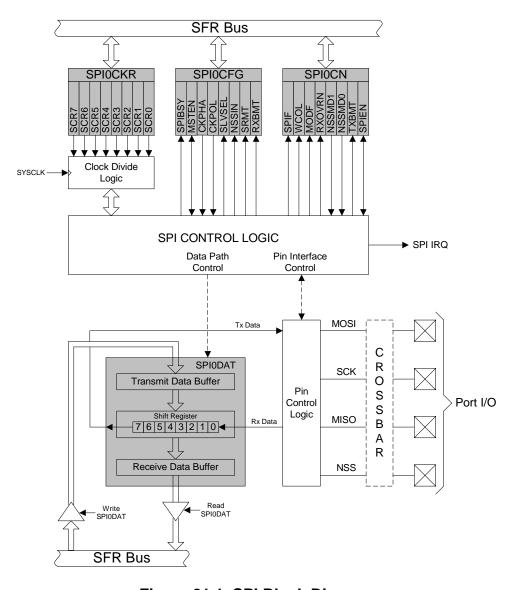
Figure 21.1. SPI Block Diagram
