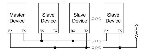
Figure 20.6. UART Multi-Processor Mode Interconnect Diagram
