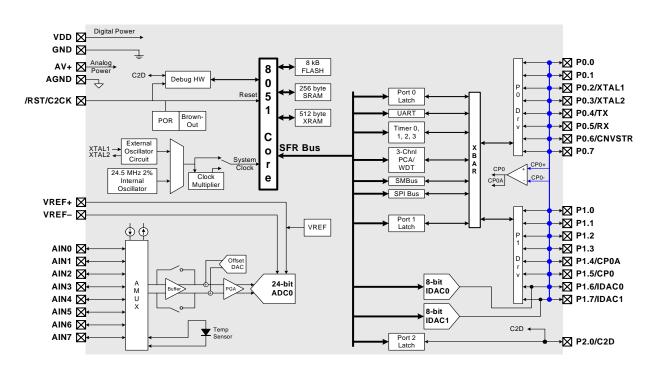
Figure 1.1. C8051F350 Block Diagram
