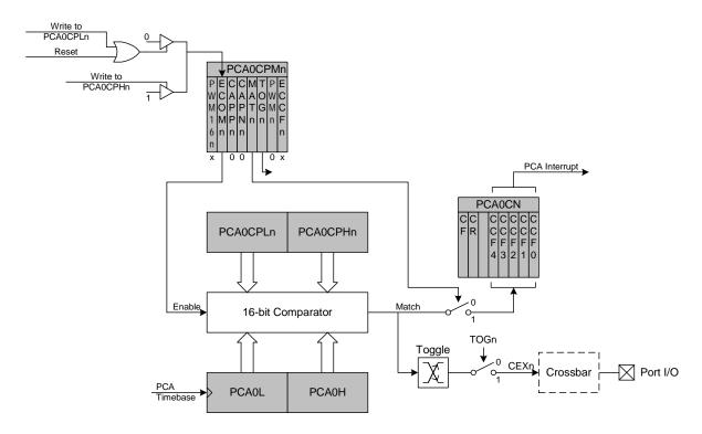
Figure 23.6. PCA High Speed Output Mode Diagram
