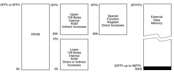
When an instruction accesses an internal location above address 7Fh, the CPU knows whether the access is to the upper 128 bytes of data RAM or to SFR space by the addressing mode used in the instruction.
