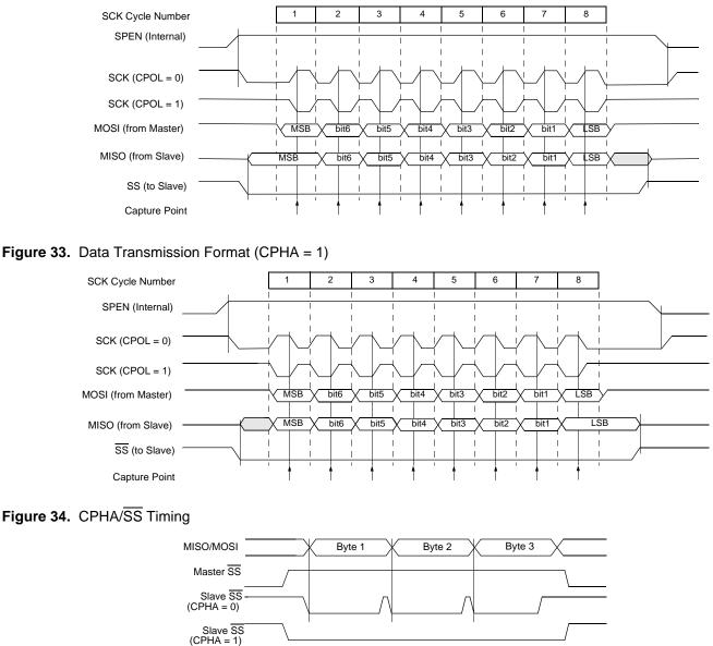
As shown in Figure 32, the first SCK edge is the MSB capture strobe. Therefore, the Slave must begin driving its data before the first SCK edge, and a falling edge on the SS pin is used to start the transmission. The SS pin must be toggled high and then low between each Byte transmitted (Figure 34).
