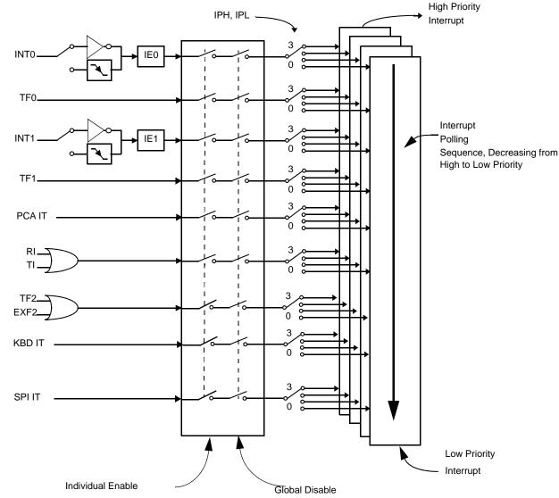
Figure 36. Interrupt Control System
