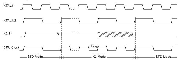
The X2 bit in the CKCON0 register (see Table 16) allows a switch from 12 clock periods per instruction to 6 clock periods and vice versa. At reset, the speed is set according to X2 bit of Hardware Security Byte (HSB). By default, Standard mode is active. Setting the X2 bit activates the X2 feature (X2 mode).
