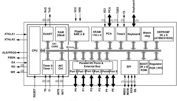
(1): Alternate function of Port 1(2): Alternate function of Port 3
