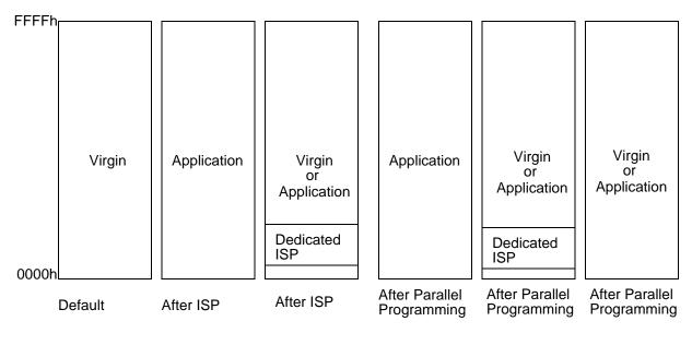
**Memory Organization** When the EA pin is high, the processor fetches instructions from internal program Flash. If the EA pin is tied low, all program memory fetches are from external memory.
