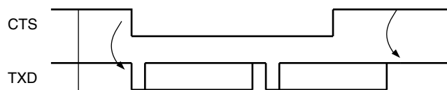
Figure 39-28. Transmitter Behavior when Operating with Hardware Handshaking
