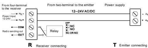
The best install height should big in 20 cm, install distance to be no smaller than 2 meters. Install should make red outside the protection equip perpendicularity to place, and is on-line at same level. Install should install first to receive part, install blast-off part again. When together at always line, receive the OFF light in the machine in order to put out, then fix, connect the line to install completion namely.
