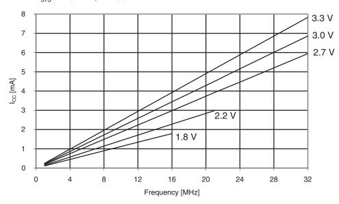
Figure 35-10. Idle Supply Current vs. Vcc
