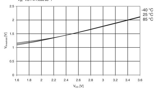
Figure 35-28. I/O Pin Input Threshold Voltage vs.  $V_{\rm CC}$
