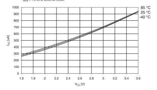
**Figure 35-4.** Active Supply Current vs. VCC  $f_{SYS} = 32.768 \text{ kHz internal } RC$
