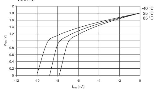
**Figure 35-22.** I/O Pin Output Voltage vs. Source Current Vcc = 3.0V
