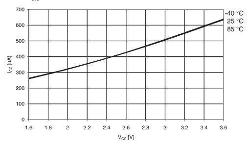
Figure 35-13. Idle Supply Current vs. Vcc
