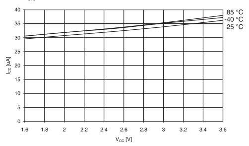
Figure 35-12. Idle Supply Current vs. Vcc
