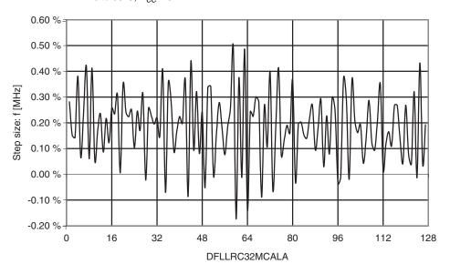
**Figure 35-38.** Internal 32 MHz Oscillator CALB Calibration Step Size T = -40 to 85°C,  $V_{CC} = 3V$
