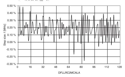
Figure 35-36. Internal 2 MHz Oscillator CALB Calibration Step Size
