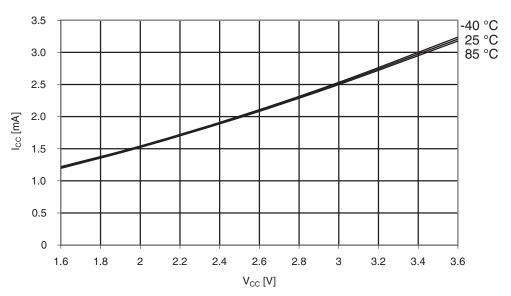
Figure 35-14. Idle Supply Current vs. Vcc
