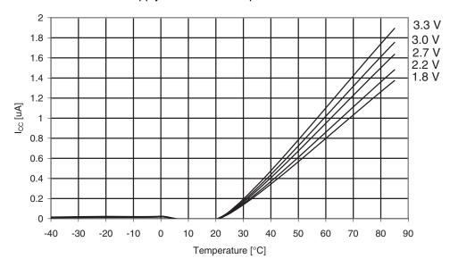
**Figure 35-16.** Power-down Supply Current vs. Temperature With WDT and sampled BOD enabled.
