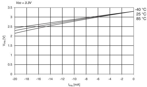
Figure 35-23. I/O Pin Output Voltage vs. Source Current
