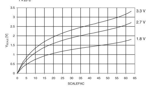
Figure 36-1. Analog Comparator Voltage Scaler vs. Scalefac  $T = 25^{\circ}C$
