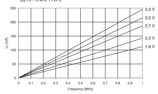
Figure 35-9. Idle Supply Current vs. Frequency
