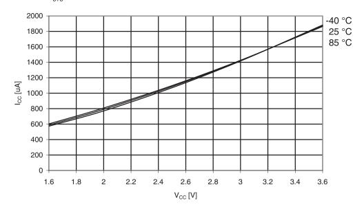
**Figure 35-6.** Active Supply Current vs. Vcc  $f_{SYS} = 32$  MHz internal RC prescaled to 8 MHz
