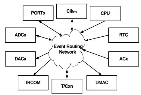
Figure 9-1. Event system block diagram.
