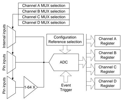
Each ADC has four MUX selection registers with a corresponding result register. This means that four channels can be sampled within 1.5 µs without any intervention by the application other than starting the conversion. The results will be available in the result registers.
