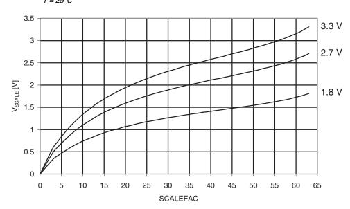
**Figure 36-3.** Analog Comparator Voltage Scaler vs. Scalefac  $T = 25^{\circ}C$
