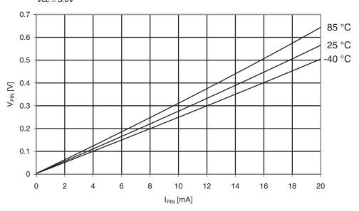
**Figure 35-26.** I/O Pin Output Voltage vs. Sink Current Vcc = 3.3V
