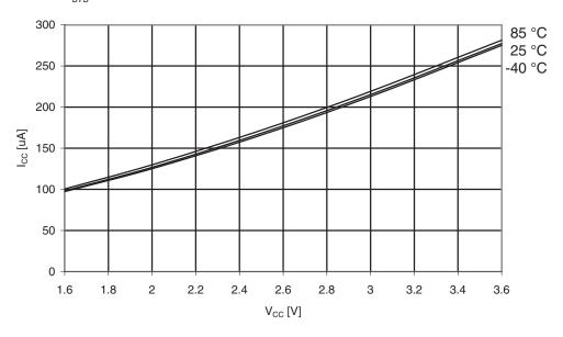
Figure 35-11. Idle Supply Current vs. Vcc
