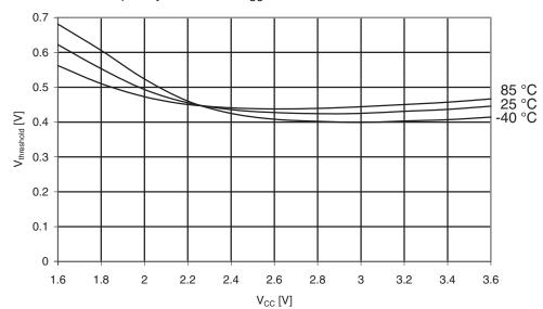
Figure 35-29. I/O Pin Input Hysteresis vs.  $V_{\text{CC}}$
