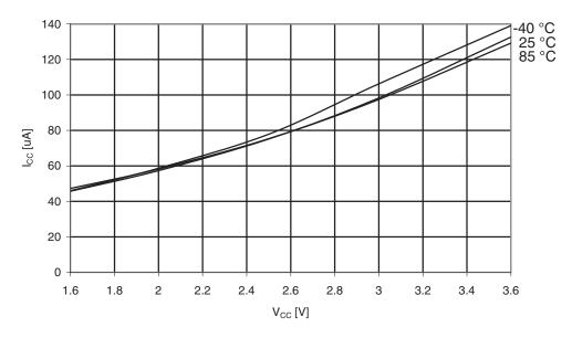
**Figure 35-5.** Active Supply Current vs. Vcc  $f_{SYS} = 2.0 \text{ MHz internal RC}$
