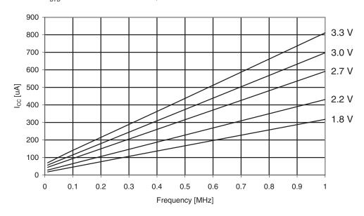
**Figure 35-2.** Active Supply Current vs. Frequency  $f_{SYS} = 1 - 32 \; MHz \; External \; clock, \; T = 25 \, ^{\circ}C$
