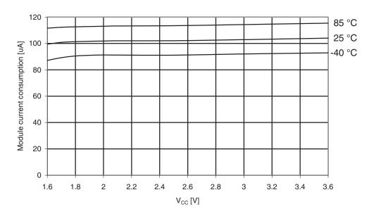
Figure 35-40. Power-up current consumption vs. Vcc
