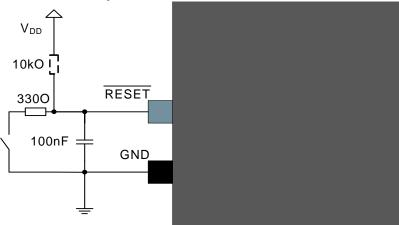
A pull-up resistor makes sure that the reset does not go low unintended causing a device reset. An additional resistor has been added in series with the switch to safely discharge the filtering capacitor, i.e. preventing a current surge when shorting the filtering capacitor which again causes a noise spike that can have a negative effect on the system.
