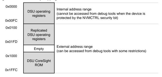
Some features not activated by APB transactions are not available when the device is protected:
