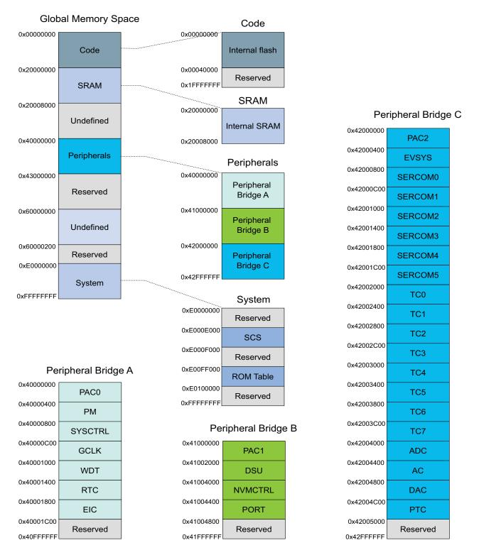
This figure represents the full configuration of the Atmel<sup>®</sup> SAM D20 with maximum flash and SRAM capabilities and a full set of peripherals. Refer to the "Configuration Summary" on page 3 for details.
