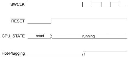
The presence of a debugger probe is detected when either Hot-Plugging or Cold-Plugging is detected. Once detected, the Debugger Present bit of the Status B register (STATUSB.DBGPRES) is set. For security reasons, Hot-Plugging is not available when the device is protected by the NVMCTRL security bit (refer to "Security Bit" on page 274).
