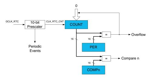
Figure 19-3. RTC Block Diagram (Mode 2 — Clock/Calendar)
