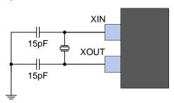
The crystal should be located as close to the device as possible. Long signal lines may cause too high load to operate the crystal, and cause crosstalk to other parts of the system.
