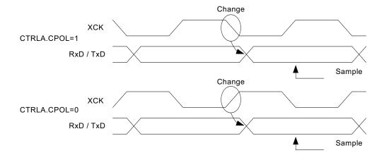
When the clock is provided through XCK (CTRLA.MODE is 0x0), the shift registers operate directly on the XCK clock. This means that XCK is not synchronized with the system clock and, therefore, can operate at frequencies up to the system frequency.
