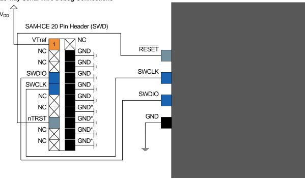
Table 34-10. 20-way Serial Wire Debug Connections (SAM-ICE)
