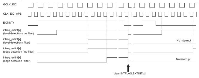
The detection delay depends on the detection mode.
