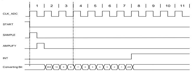
Figure 29-7. ADC Timing for Free Running in Single-Ended Mode without Gain
