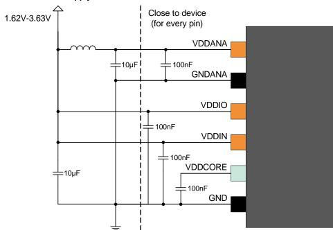
Table 34-1. Power Supply Connections,  $V_{\text{DDCORE}}$  From Internal Regulator
