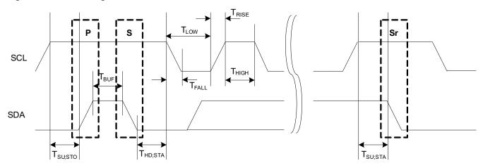
The following parameters are timed using the SCL low time period. This comes from the Master Baud Rate Low bit group in the Baud Rate register (BAUD.BAUDLOW) when non-zero, or the Master Baud Rate bit group in the Baud Rate register (BAUD.BAUDL) when BAUD.BAUDLOW is zero.
