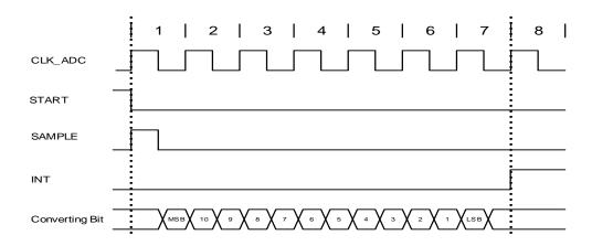
Figure 29-4. ADC Timing for One Conversion in Differential Mode without Gain, but with Increased Sampling Time
