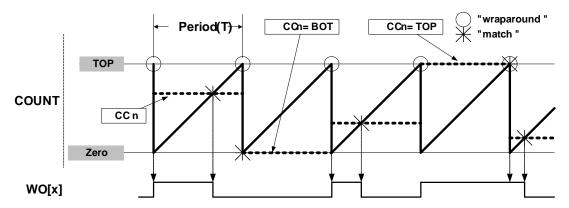
In match operation, Compare/Capture register CC0 is used as the top value, and in this case WO[0] will toggle on every overflow/underflow.
