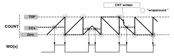
When MFRQ is used, the value in CC0 will be used as the top value and WO[0] will toggle on every overflow/underflow.
