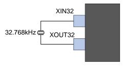
Crystals specifying load capacitance (CL) higher than TBDpF, require external capacitors applied as described in Figure 34-8.
