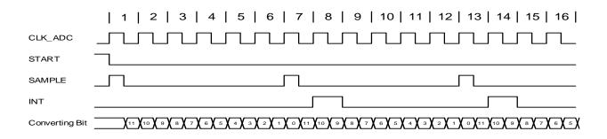
Figure 29-6. ADC Timing for One Conversion in Single-Ended Mode without Gain
