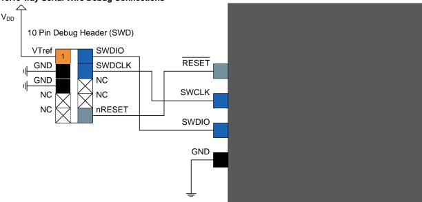
For debuggers/programmers that support the 10-way ARM debug interface should be connected as shown in Figure 34-10 with details described in Table 34-9.
