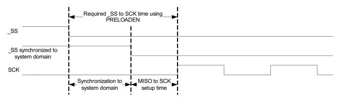
Only one data character written to DATA will be preloaded into the shift register while the synchronized \_SS signal (see Figure 26-4) is high. The next character written to DATA before \_SS is pulled low will be stored in DATA until transfer begins. If the shift register is not preloaded, the current contents of the shift register will be shifted out.
