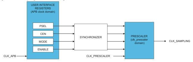
Figure 17-2. Sampling Mode Block diagram
