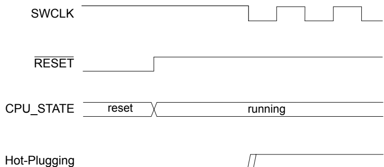
Figure 13-3. Hot-Plugging Detection Timing Diagram
