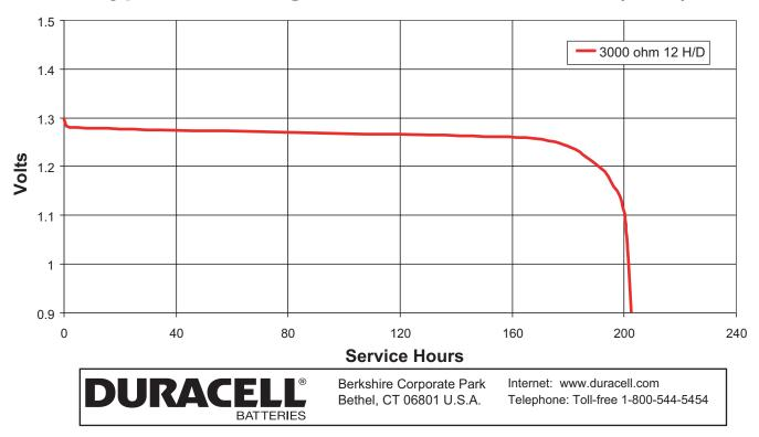
\* Delivered capacity is dependent on the applied load, operating temperature and cut-off voltage. Please refer to the chart and discharge data shown for examples of the energy / service life that the battery will provide.
