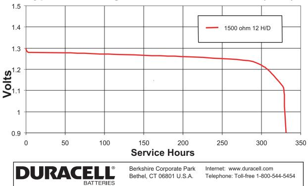
\* Delivered capacity is dependent on the applied load, operating temperature and cut-off voltage. Please refer to the chart and discharge data shown for examples of the energy / service life that the battery will provide.
