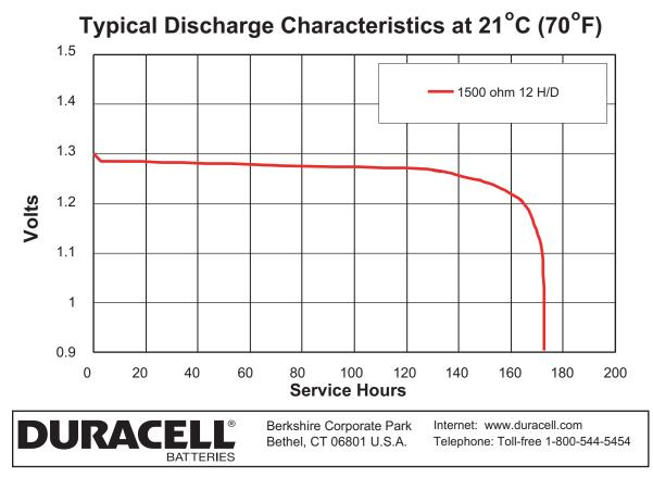
\* Delivered capacity is dependent on the applied load, operating temperature and cut-off voltage. Please refer to the chart and discharge data shown for examples of the energy / service life that the battery will provide.
