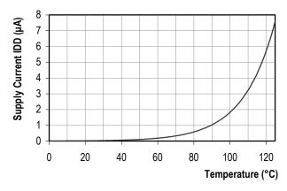
**Figure 6** Dependency of supply current (sleep mode) versus temperature at VDD = 3.0V. Please note the variance of the displayed data may exceed ±25%.
