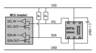
**Figure 11** Typical application circuit, including pull-up resistors R<sub>P</sub> and decoupling of VDD and VSS by a capacitor.
