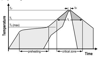
**Figure 9** Soldering profile according to JEDEC standard.  $T_P \le 260^{\circ}\text{C}$  and  $t_P \le 30\text{sec}$  for Pb-free assembly.  $T_L \le 220^{\circ}\text{C}$  and  $t_L \le 150\text{sec}$ . Ramp-up/down speeds shall be  $\le 5^{\circ}\text{C/sec}$ .
