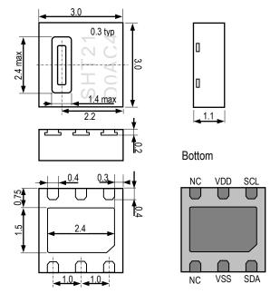
**Figure 1:** Drawing of SHT25 sensor package, dimensions are given in mm (1mm = 0.039inch), tolerances are  $\pm 0.1$ mm. The die pad (center pad) is internally connected to VSS. The NC pads must be left floating. VSS = GND, SDA = DATA. Numbering of E/O pads starts at lower right corner (indicated by notch in die pad) and goes clockwise (compare Table 2).
