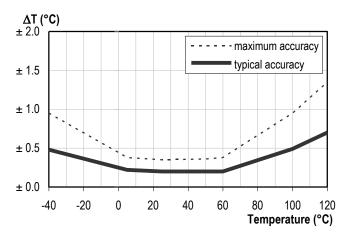
Figure 3 Maximal tolerance for temperature sensor in °C.
