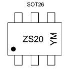
ZS20 = Product Type Marking Code YM = Date Code Marking Y or  $\overline{Y}$  = Year (ex: C = 2015) M or  $\overline{M}$  = Month (ex: 9 = September)
