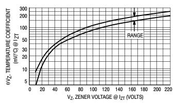
Figure 3. Temperature Coefficient-Range for Units 10 to 220 Volts
