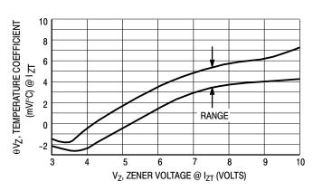
Figure 2. Temperature Coefficient-Range for Units 3 to 10 Volts
