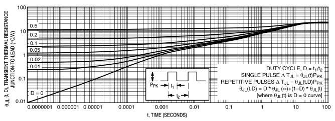
Figure 4. Typical Thermal Response L, Lead Length = 3/8 Inch
