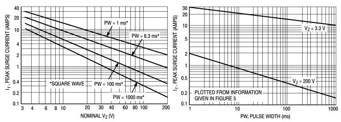
Figure 5. Maximum Non-Repetitive Surge Current versus Nominal Zener Voltage (See Note 4)
