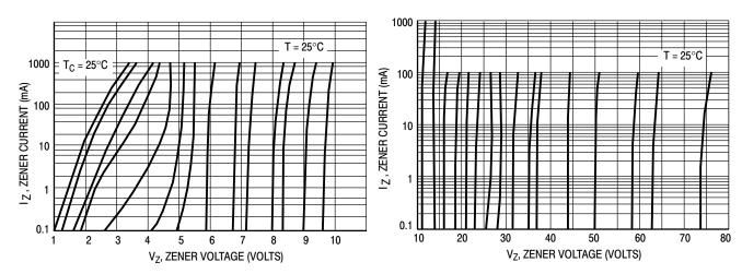
Figure 7. Zener Voltage versus Zener Current  $V_Z = 3.3 \text{ thru } 10 \text{ Volts}$
