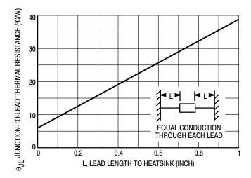
Figure 1. Typical Thermal Resistance
