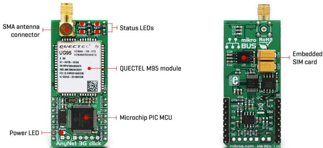
There are four LEDs used to display the connection status. Before the connection and communication with the AWS is possible, the setup procedure must be followed. For detailed step by step information, refer to the setup manual.
