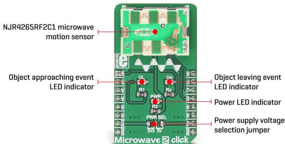
The integrated MCU of the NJR4265RF2C1 module processes the signal reduces the noise and enhances the useful signal, allowing reliable detection and steady sensing of the movement. It then makes a movement direction decision, based on the collected data and signals it back to the host MCU.
