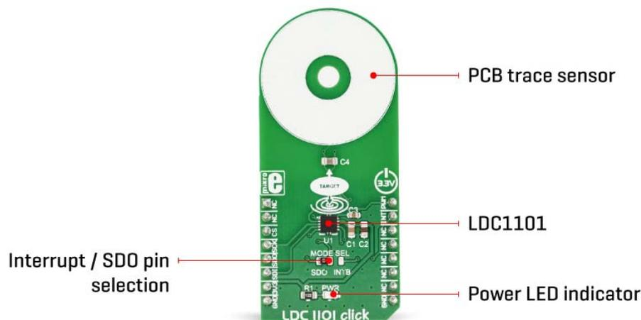
Two sensing cores work independently. One core offers a fast impedance and inductance (RP+L) readings with 16-bit resolution, while the other core offers high-resolution 24-bit readings of the inductance (LHR). While the RP+L is capable of running without the input clock, the LHR mode requires a clock signal at the CLKIN pin. Therefore, the CLKIN pin is routed to the mikroBUS™ PWM pin. Without the valid clock at this pin, the LHR mode will not be available.
