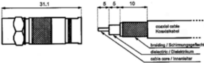
1. Strip the cable in a way, until app. 5-10 mm of the inner conductor, app. 5-10 mm dielectric and app. 10 mm of the shielding are visible.
